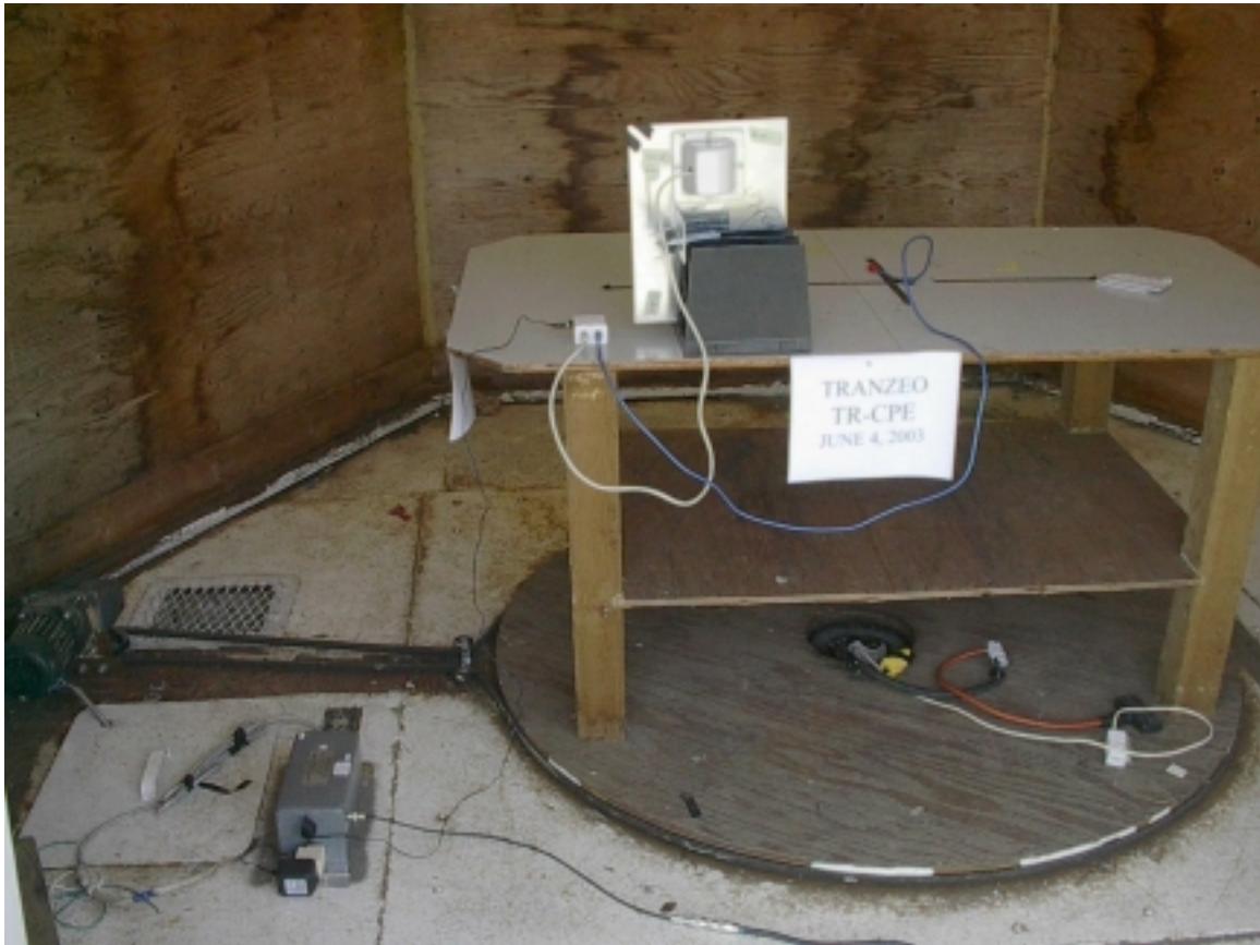
Conducted Emissions Setup
