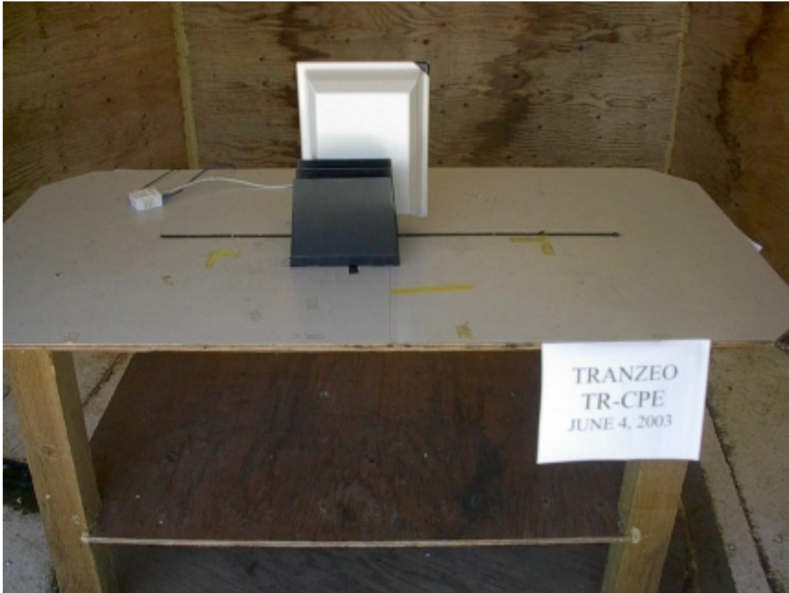
Front Emissions Test Setup
