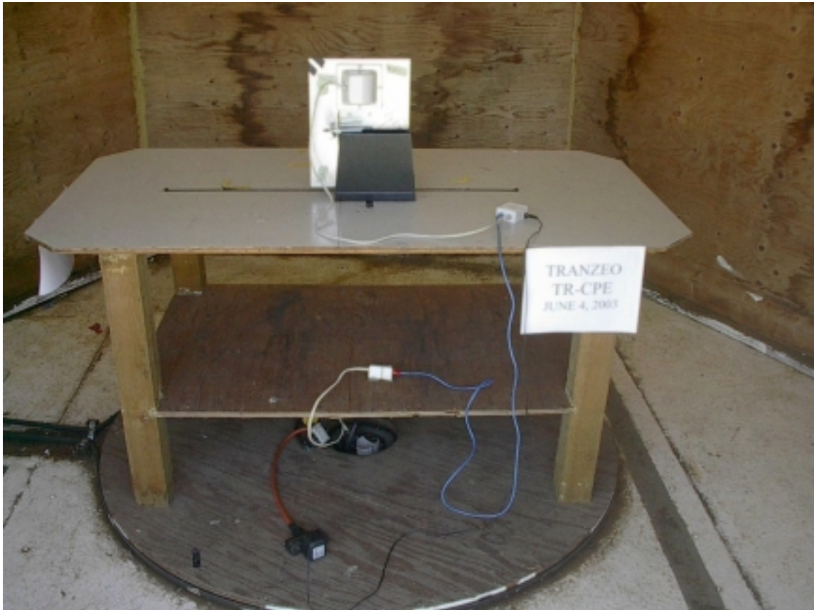
Rear Emissions Test Setup
