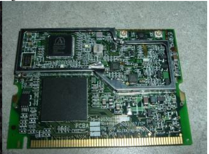
Figure 4 – Radio card without rf shield
