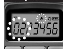
If your ID is called on the current channel, the radio will be switched to the calling mode and the icon "█" will be indicated on the LCD. You will hear an audible tone for 2 seconds. The radio's ID that you are transmitting will be on the LCD, and the first two numbers of memory will be also flashing if the ID is already assigned in the 5TONE memories.
