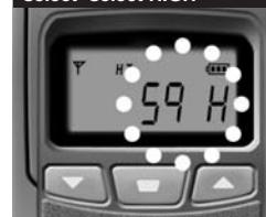
Press the "F" button once to select Squelch system, the icon "59" will begin flashing. This is a sensitivity adjustment function for users to communicate at the most comfortable situation. Select Low/High using the Up/Down buttons, it'll be then stored automatically at the same time. If no buttons are pressed in 5 seconds after selecting functions, the monitor will switch back to the main display. Press the PTT button to finish the function mode.
