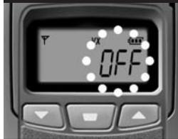
Select the VOX Mode by pressing the "F" button 7 times, the icon "VX" will begin flashing. Select On/Off with the Up/Down buttons, it'll be then stored automatically at the same time. If no buttons are pressed in 5 seconds after selecting functions, the display will switch back to the main display. Press the PTT button to finish the function mode.
