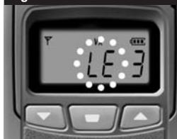
Select the VOX Mode by pressing the "F" button 8 times, the icon "LEV" will begin flashing and be indicated on the LCD. Sensitivity is how loud you have to talk to activate the VOX circuit. The VOX has 9 levels of sensitivity that can be selected using the Up/Down buttons. Option will require more voice level to activate, it'll be useful in very noisy areas. Select the VOX level desired, and press the PTT button to save it.
