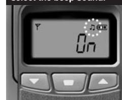
This function helps you confirm that you press the buttons properly with the beep sound. Press the "F" button twice to select the beep sound, the icon " " will begin flashing. Select On/Off using the Up/Down buttons, it'll be then stored automatically at the same time. If no buttons are pressed in 5 seconds after selecting functions, the display will switch back to the main display. Press the PTT button to finish the function mode.
