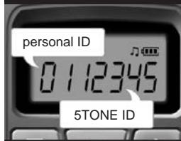
You can change the 5TONE Calling Mode by pressing the "F" button for over 2 seconds, and switch to the general calling channel by pressing it one more time. You can use the 5TONE Calling Mode only when you input your personal ID and 5TONE ID. You can communicate with other specified radios or with the members of same group without any external interference, and also can call someone's radio that you know his/her 5TONE ID.
