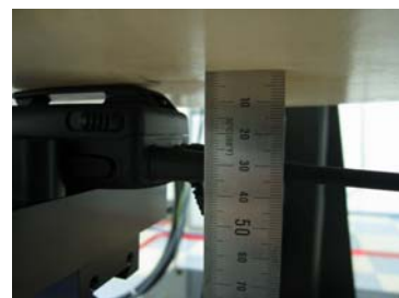
Figure 12. Body SAR Test Setup
