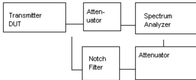
Method of Measuring Conducted Spurious Emissions
