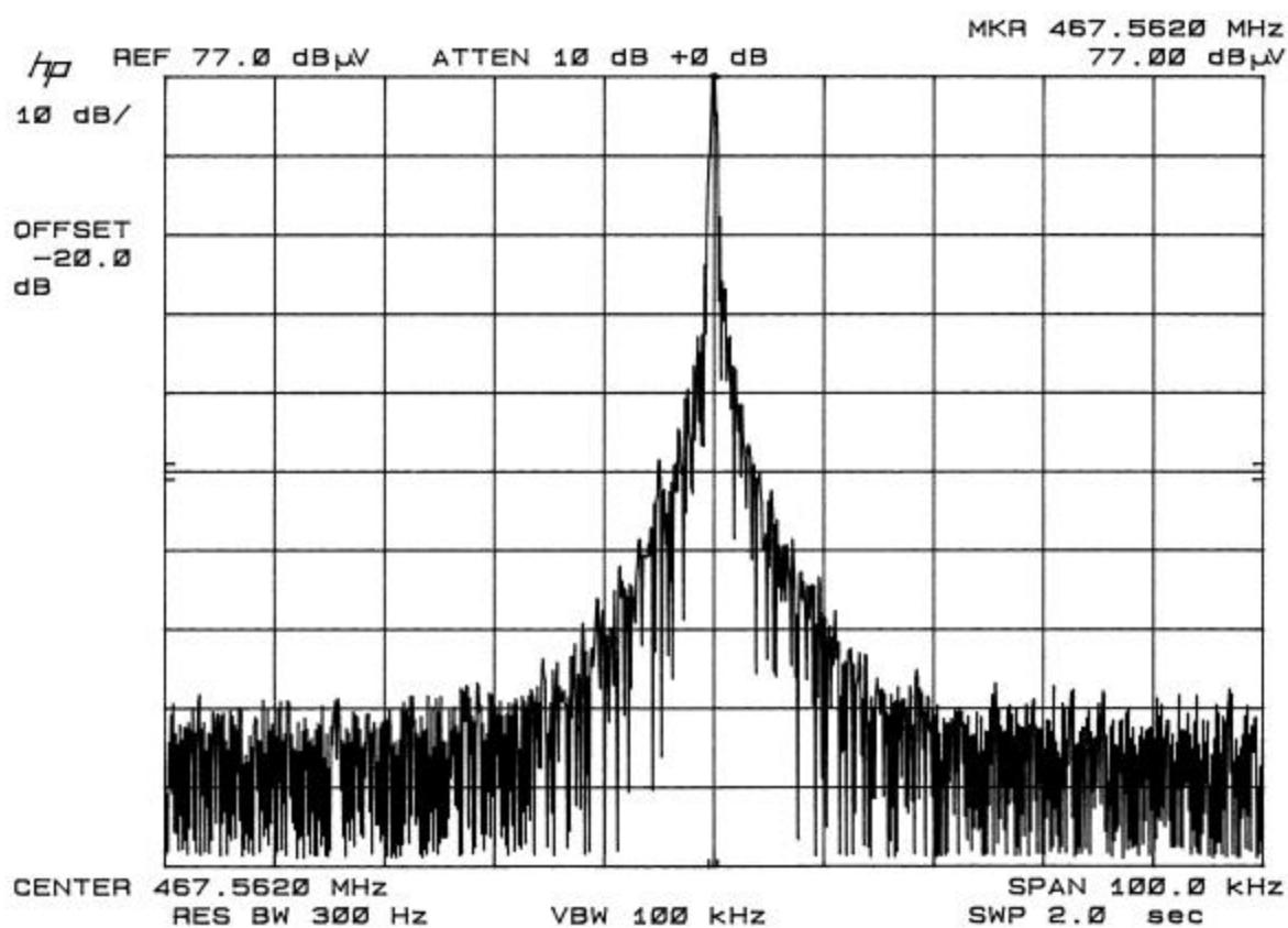
2.1051 Spurious emissions at antenna terminals (conducted):
