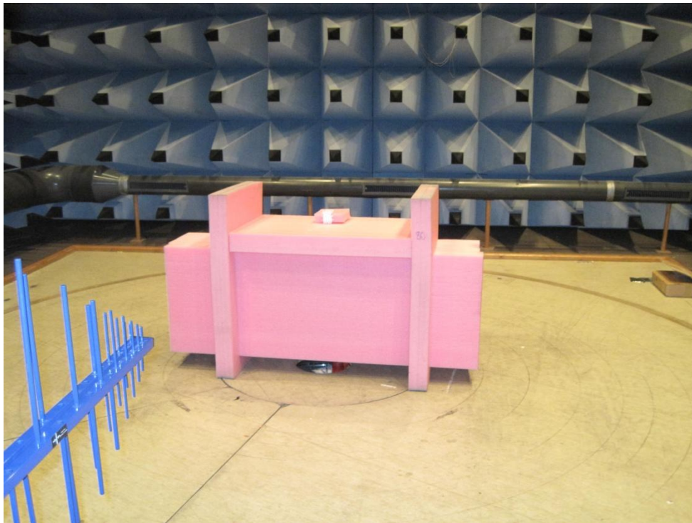
Photo 4.2.1 Test setup regarding measurement of radiated limits below 1 GHz.
