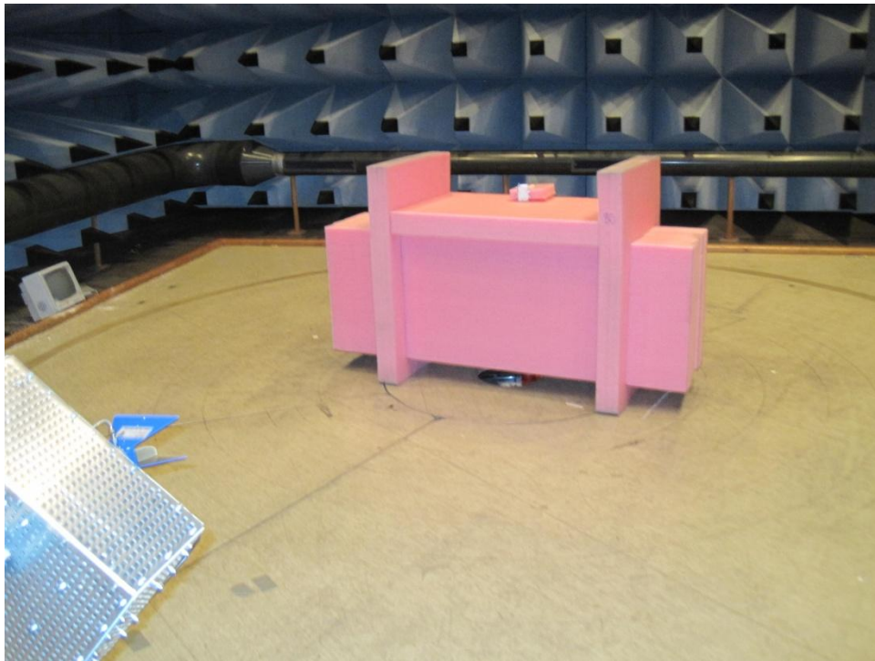
Photo 4.3.1 Test setup regarding measurement of radiated limits above 1 GHz.
