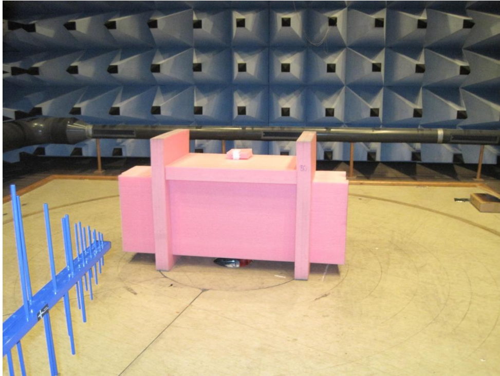
Photo 4.8.1 Test setup regarding measurement of field strength of the fundamental.
