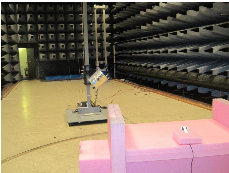
Photo 4.3.2 Test setup regarding measurement of radiated limits above 1 GHz.
