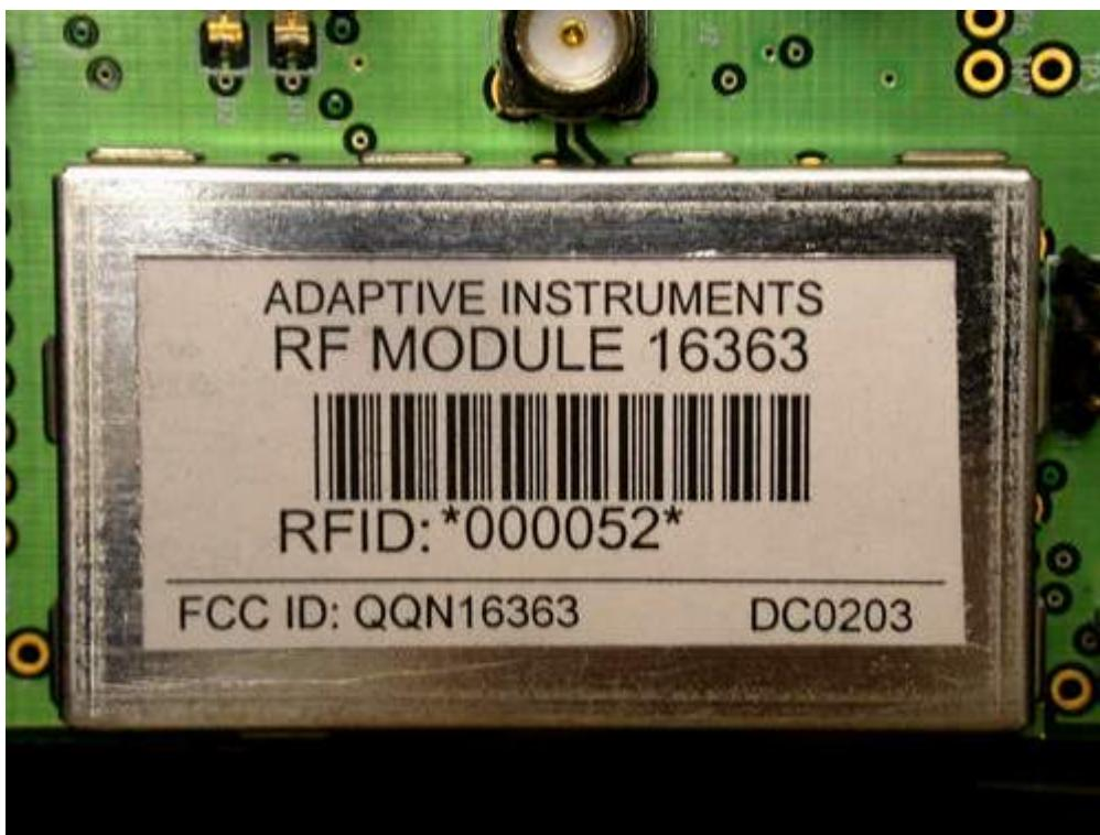
The enclosure of the product that uses this module also must have a label referring to the enclosed module as well as the exact paragraph shown below. An example is shown in the following pictures.
