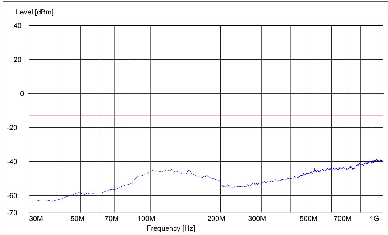
**RADIATED SPURIOUS EMISSIONS****Tx @ 1851.25MHz: 30MHz - 1GHz**
