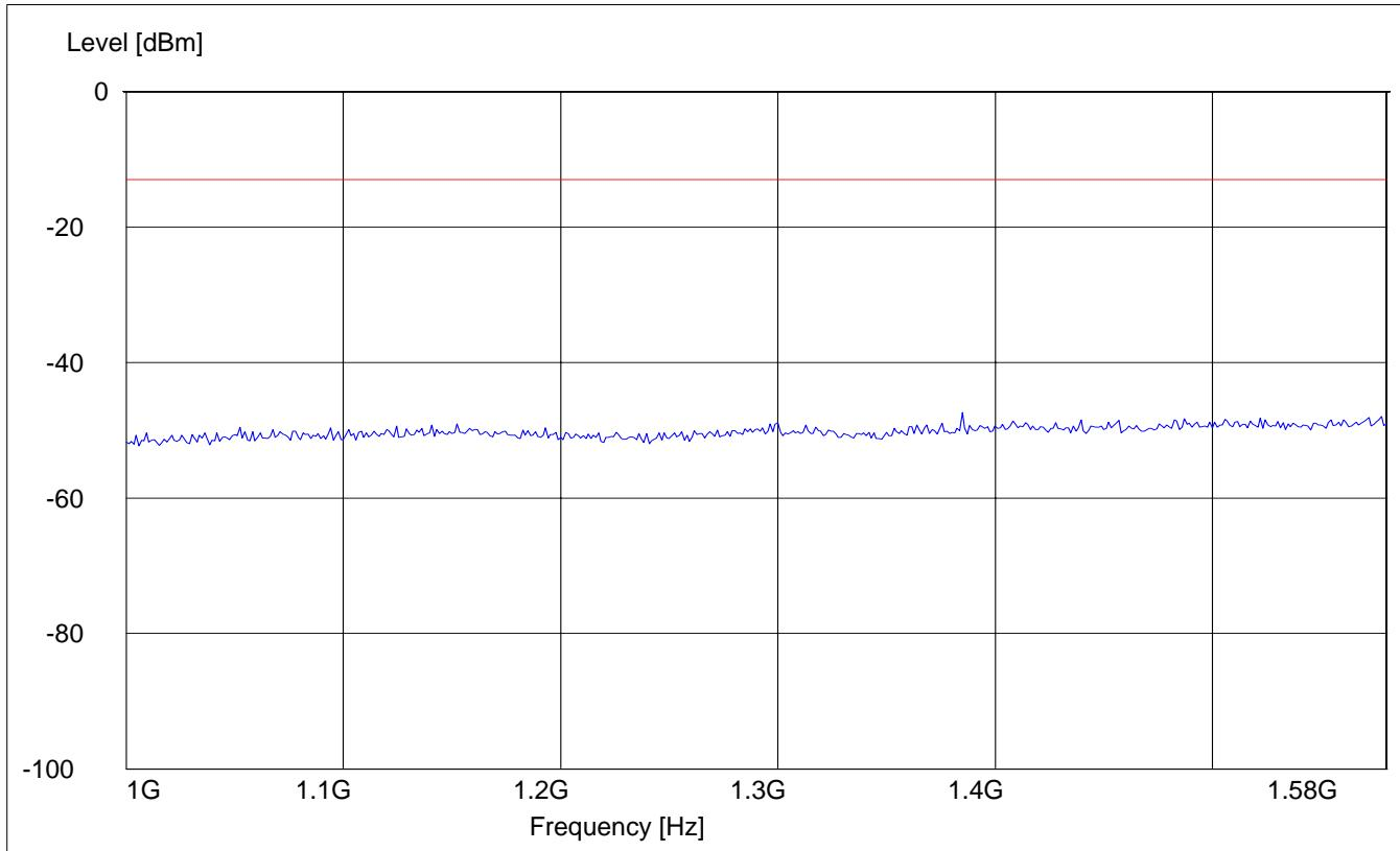
**RADIATED SPURIOUS EMISSIONS (GSM-850)****Tx @ 847.75MHz: 1.58GHz – 3GHz**
