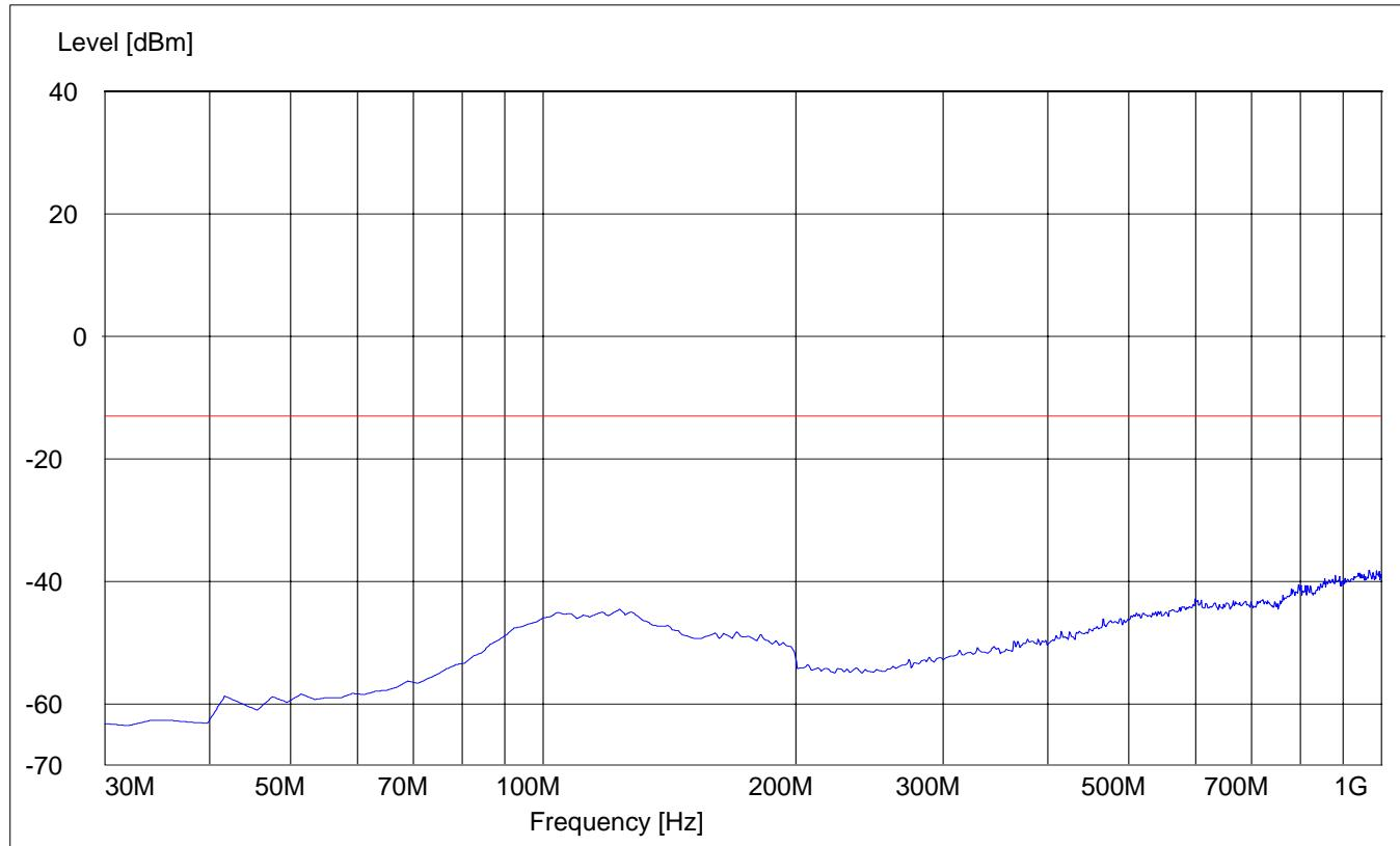
**RADIATED SPURIOUS EMISSIONS (IDLE MODE)****Antenna: horizontal****EUT in Idle Mode: 30MHz – 1GHz**
