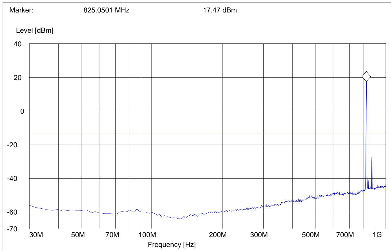
**RADIATED SPURIOUS EMISSIONS (GSM-850)****Tx @ 825.25MHz: 1GHz – 1.58GHz**
