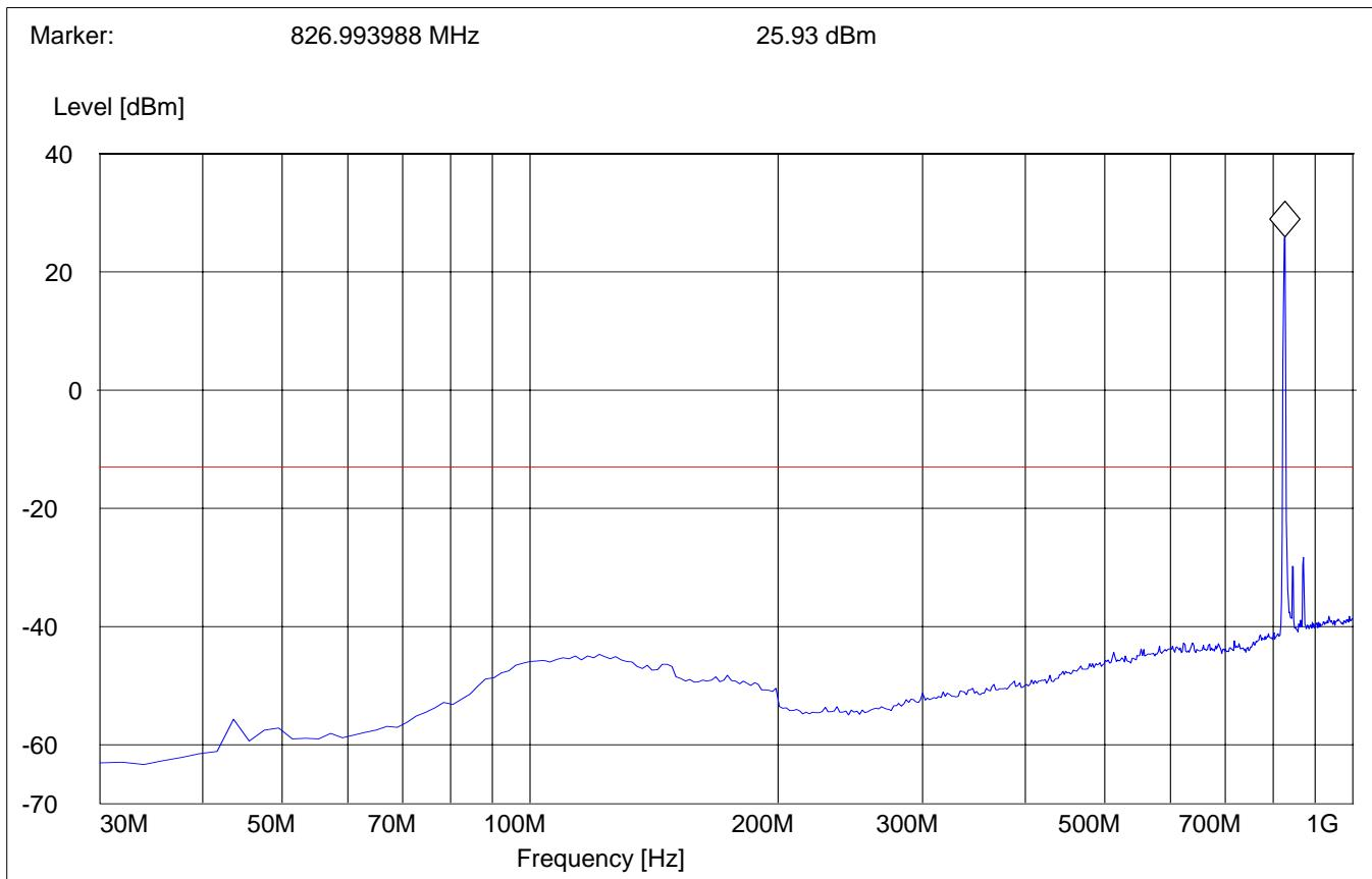
**RADIATED SPURIOUS EMISSIONS (GSM-850)****Tx @ 825.25MHz: 30MHz - 1GHz**
