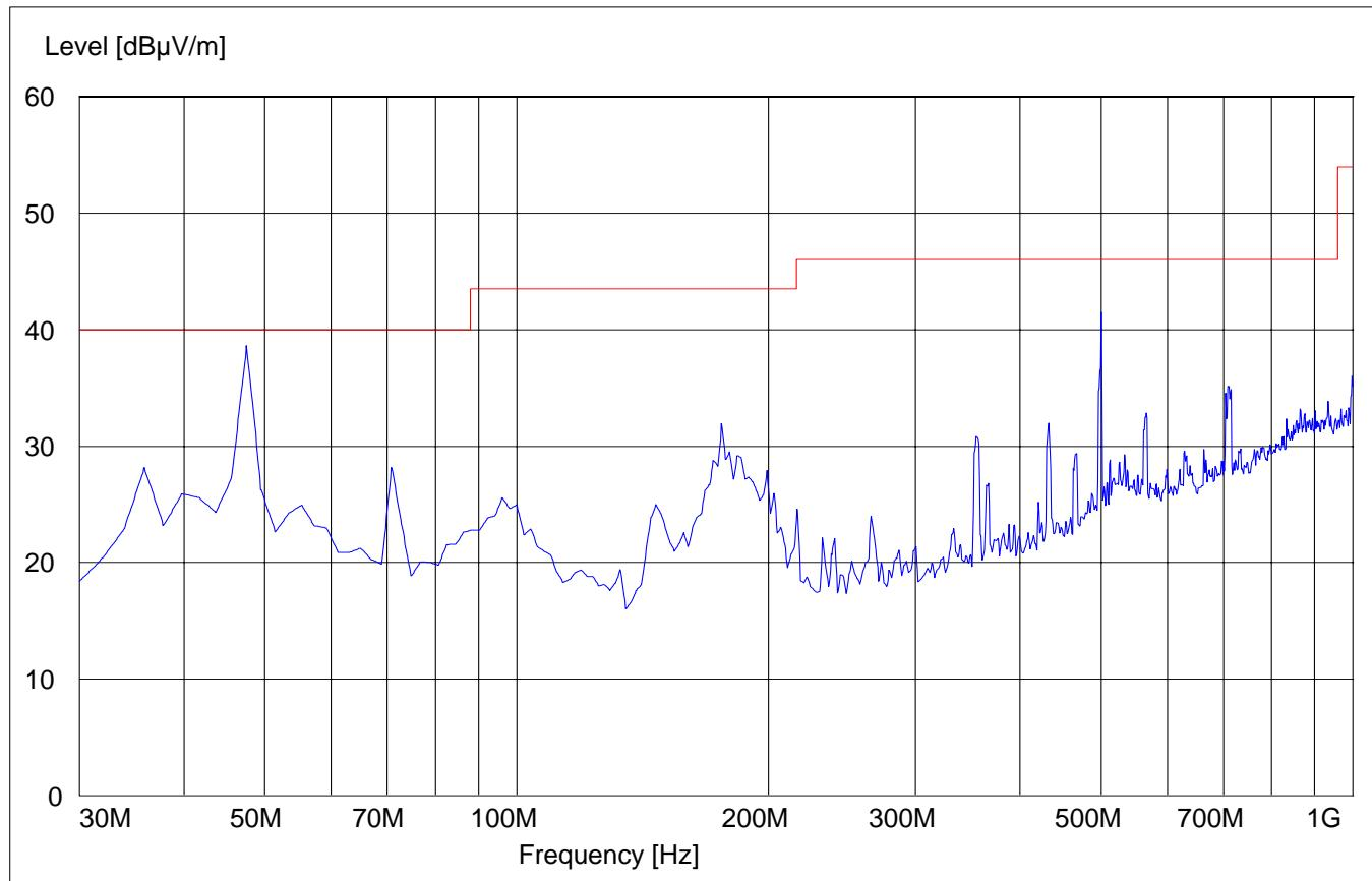
**RECEIVER RADIATED EMISSIONS****EUT in Idle Mode: 30MHz – 1GHz****Antenna: horizontal****SWEEP TABLE: "FCC Spur 30M-1G"**
