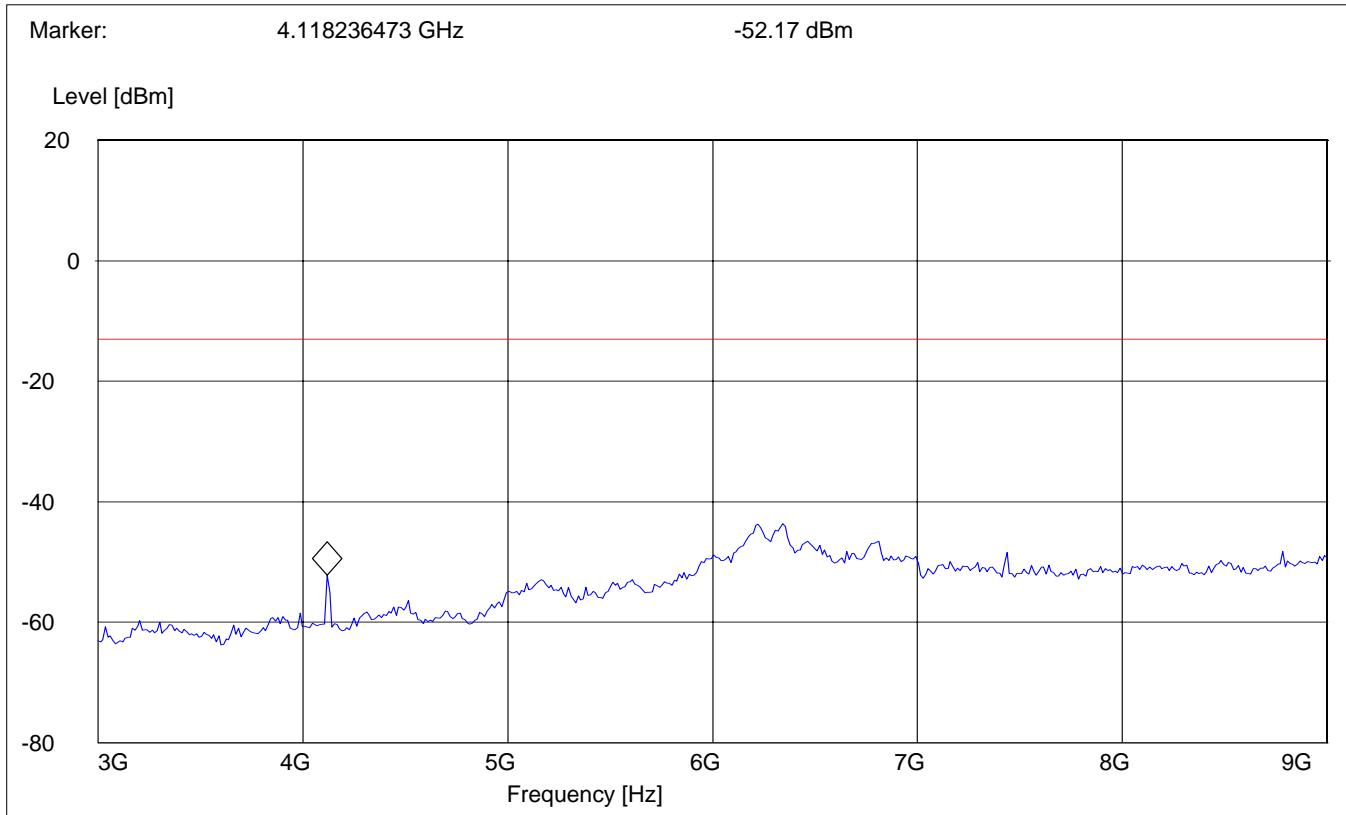
**RADIATED SPURIOUS EMISSIONS (GSM-850)****Tx @ 836.5MHz: 1GHz – 1.58GHz**
