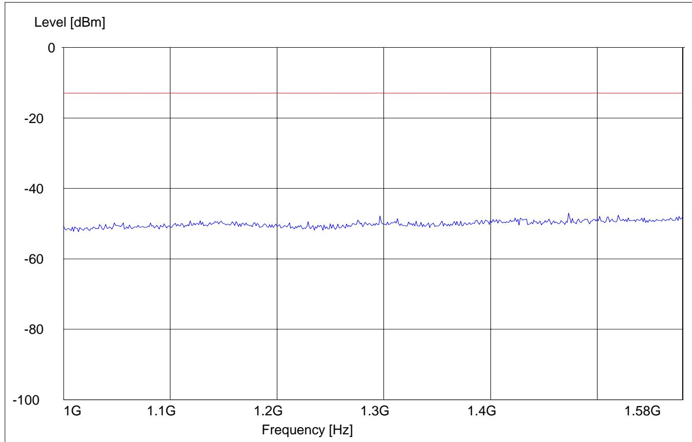
**RADIATED SPURIOUS EMISSIONS (GSM-850)****Tx @ 836.5MHz: 1.58GHz – 3GHz**
