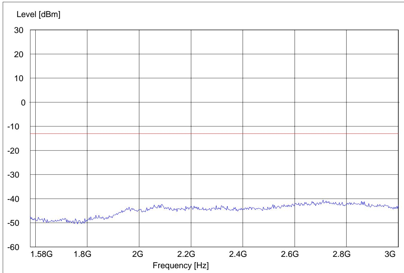
**C3311 (PinPoint CDMA)****RADIATED SPURIOUS EMISSIONS (GSM-850)****Tx @ 825.25MHz: 1GHz – 1.58GHz**
