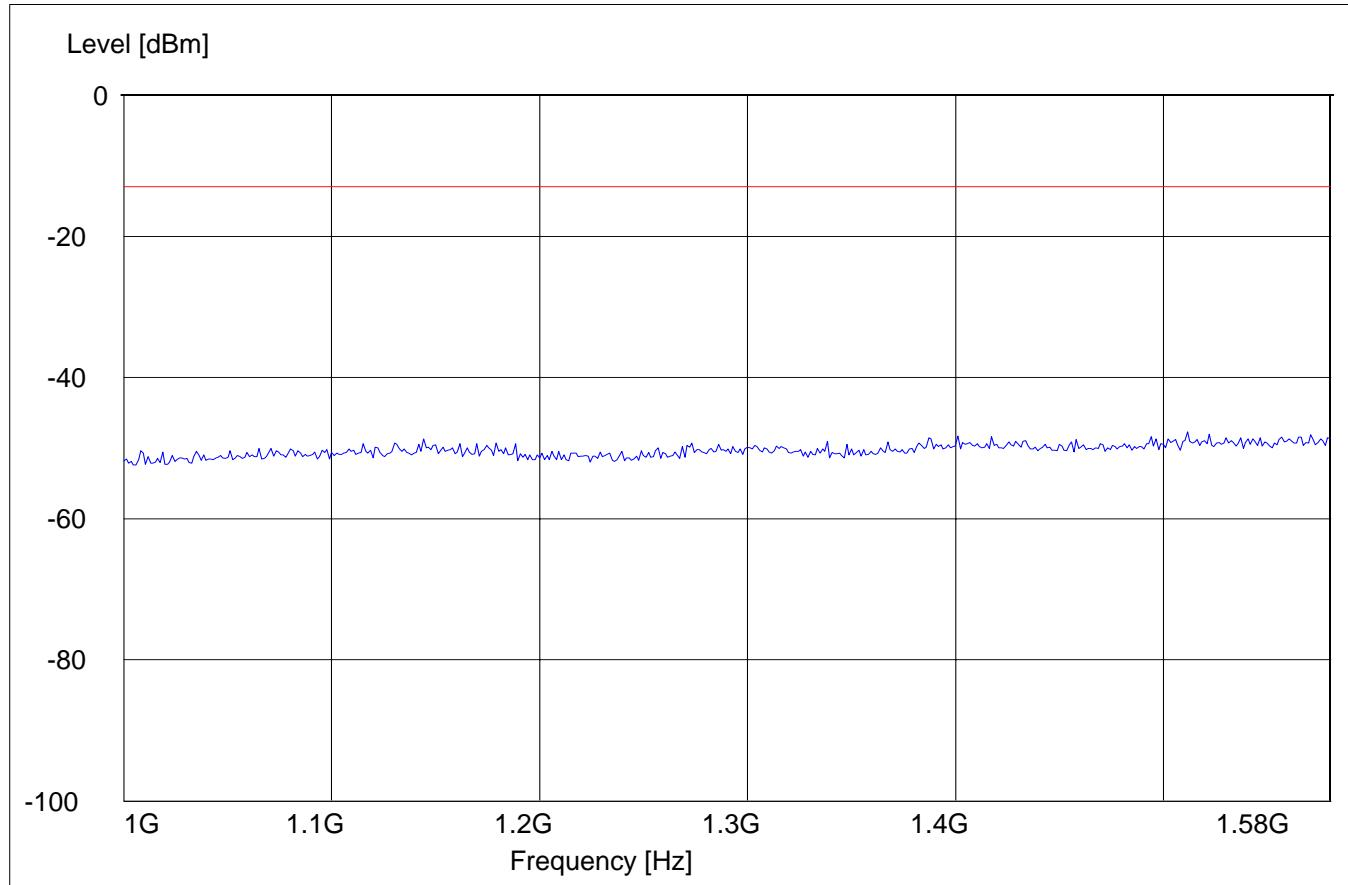
**RADIATED SPURIOUS EMISSIONS (GSM-850)****Tx @ 847.75MHz: 1.58GHz – 3GHz**
