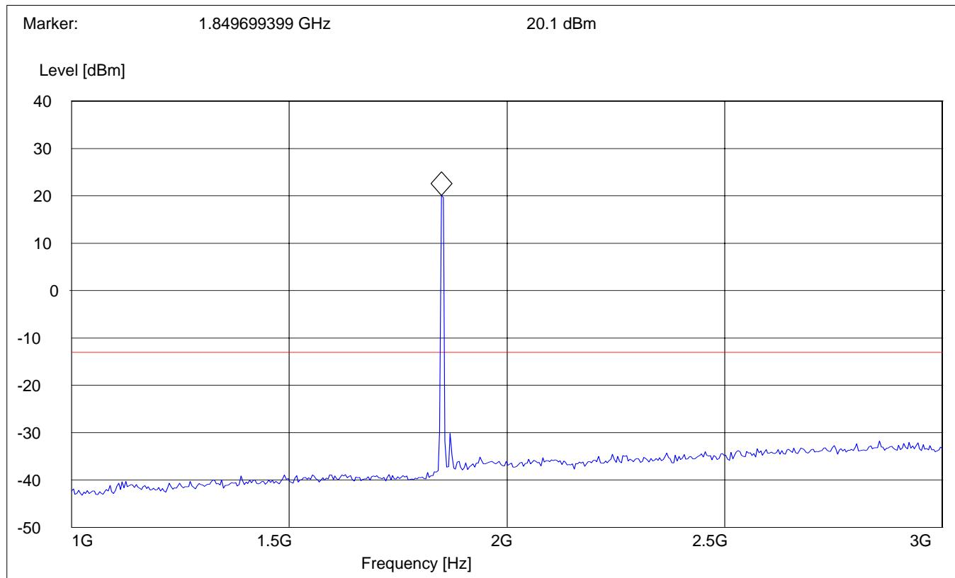
**RADIATED SPURIOUS EMISSIONS****Tx @ 1851.25MHz: 3GHz – 18GHz**
