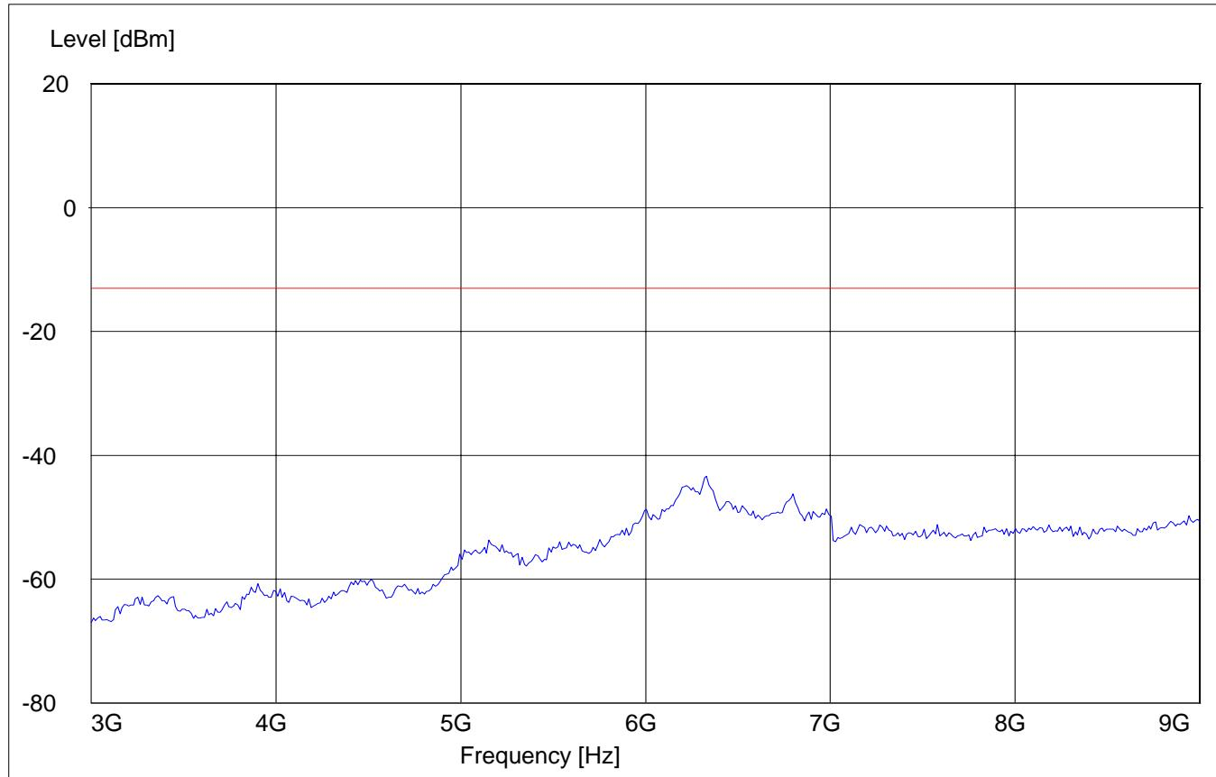
**RADIATED SPURIOUS EMISSIONS (GSM-850)****Tx @ 836.5MHz: 1GHz – 1.58GHz**
