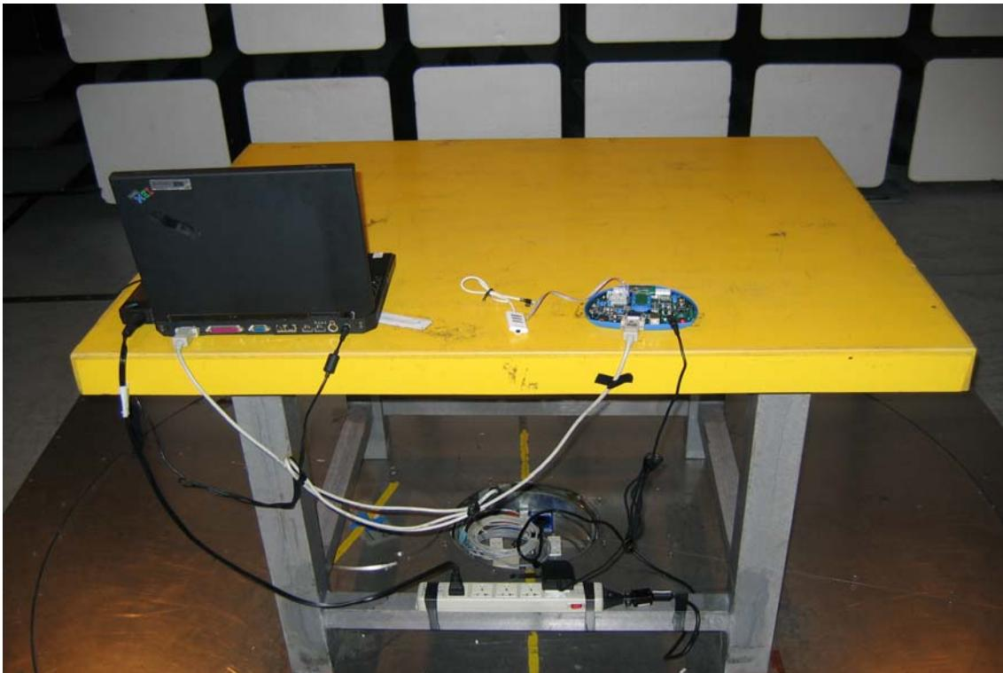
**Radiated Emission Set up Photos (Audio-in Mode)**
