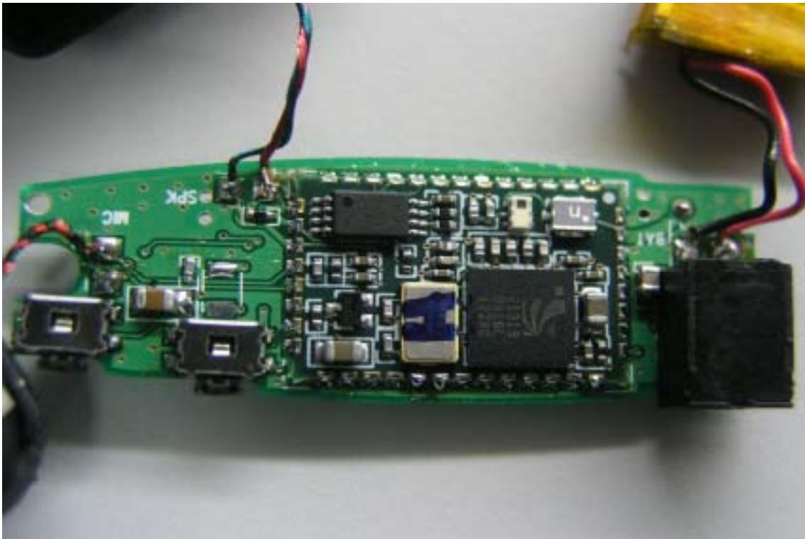
*Internal of EUT (Model: PBHFABH2C2-X ; ET2000R ; BTH3R ;BTH4R)*
