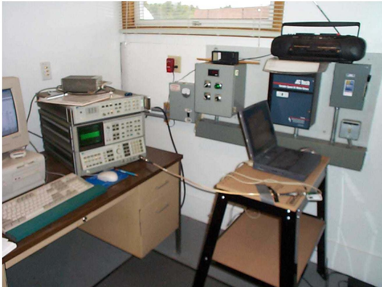
Intentional Radiator Conducted Emissions (Directly connected to the Spectrum Analyzer) Testing
