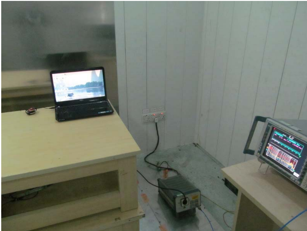
FCC RADIATED EMISSION TEST SETUP
