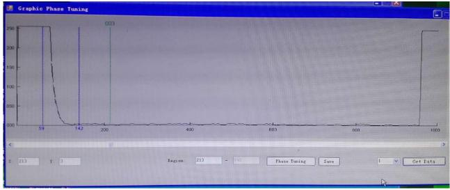
Choose channel [1] or [2] or [3]; click GET DATA to slide the mouse green line, and the green line position data will automatically fill in REGION [], point Phase Tuning and then point GET DATA to adjust the curve will appear, repeat the above two steps until satisfactory; finally point SAVE saves PHASE into memory.
