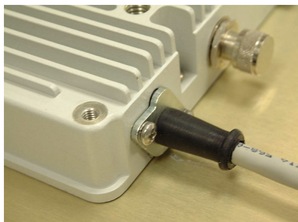
Figure 2-7: Cable connection to Outdoor Unit
