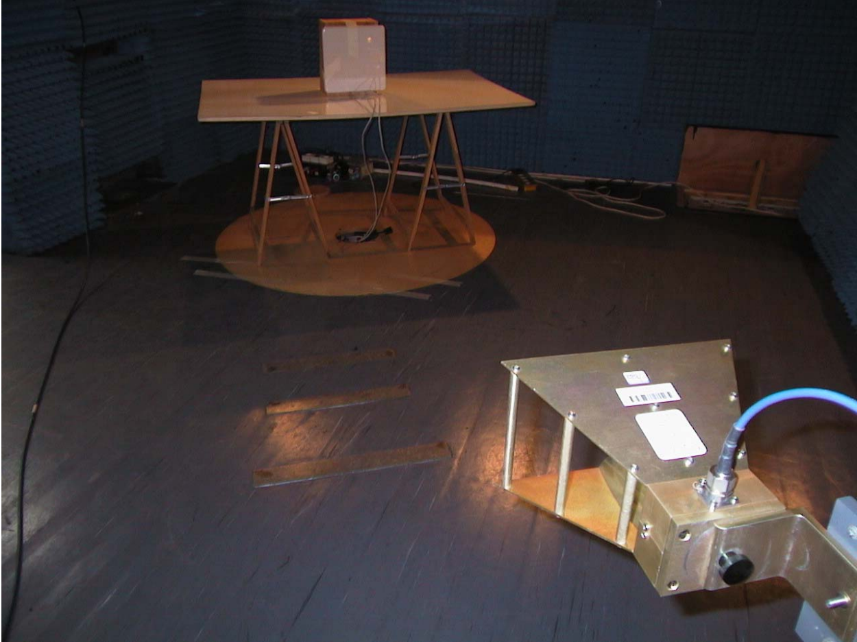
Radiated emission 1GHz – 18GHz Setup
