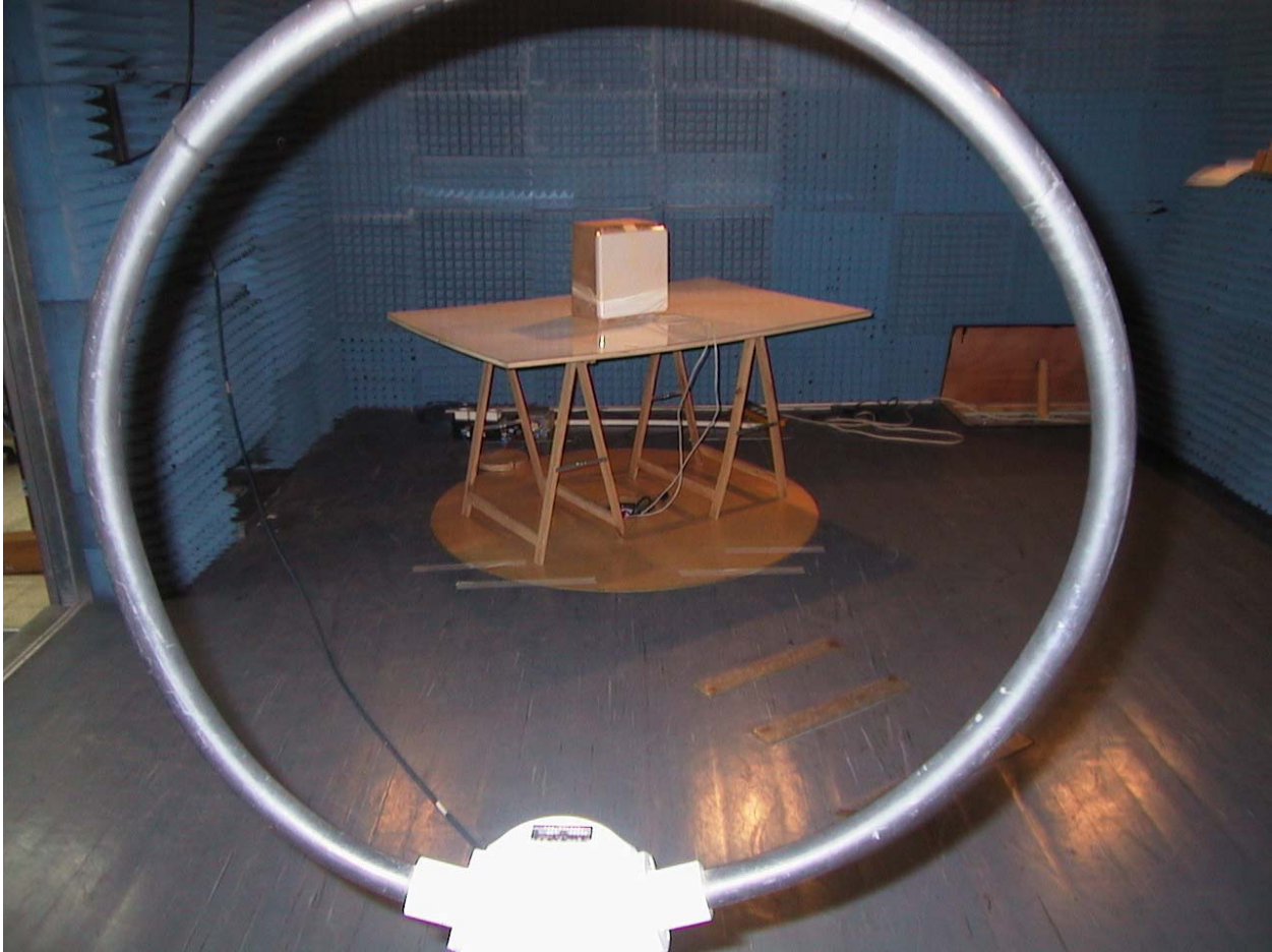
Radiated emission up to 30MHz Setup
