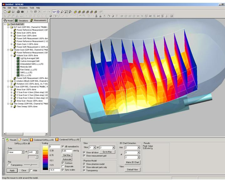
Display of results (3D Volume Scan) from the superposition of measured data in the viewer.
