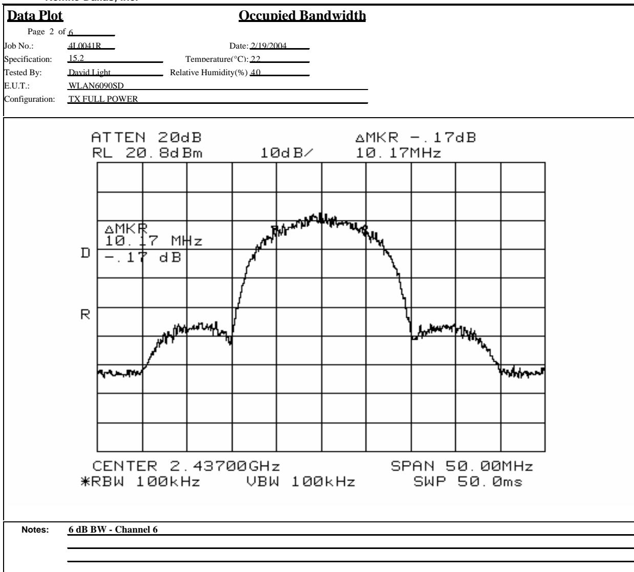
EQUIPMENT: WLAN6090SDREPORT NO.: 4L0041RUS1**Test Data – Occupied Bandwidth**
