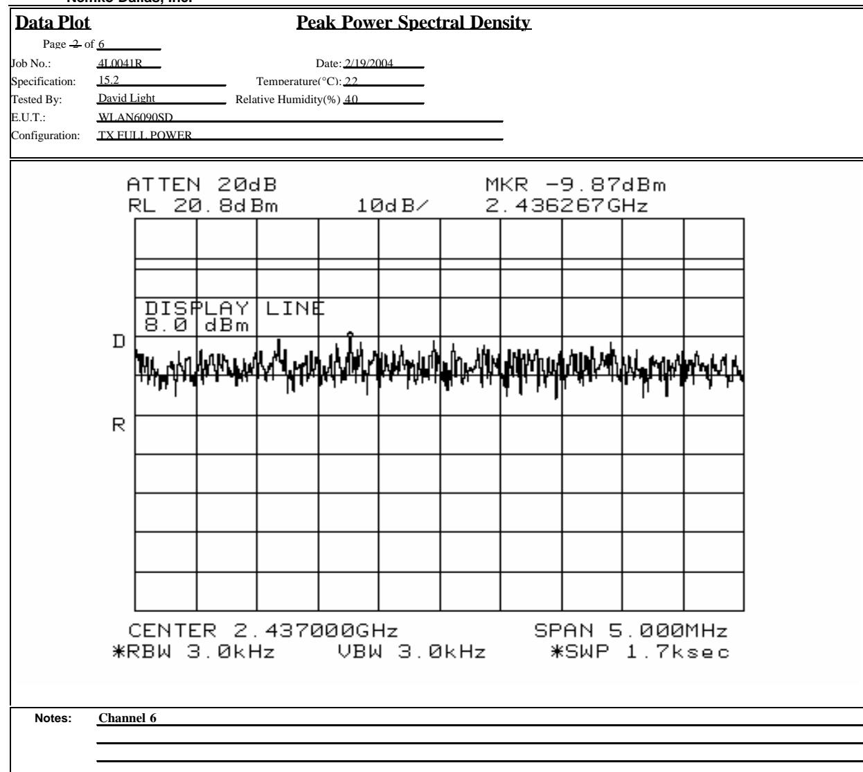
**Test Data – Peak Power Spectral Density**
