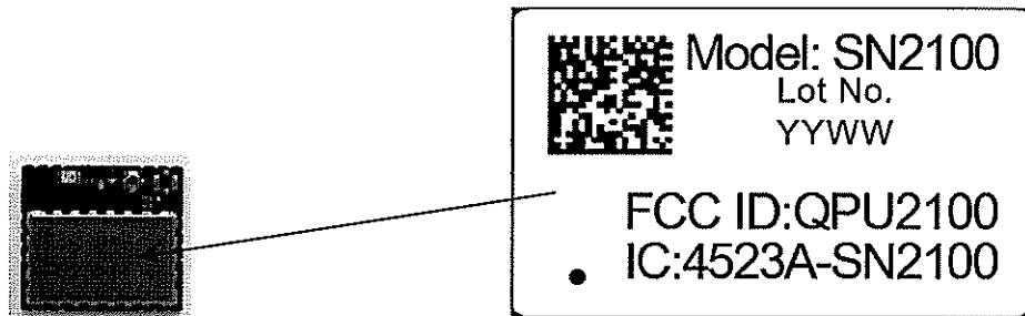
Label is printed and permanently affixed to shield or laser marked directly into shield.
