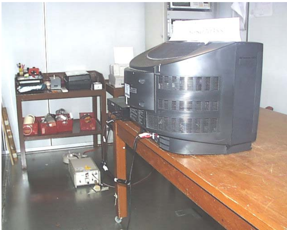
Conducted Emissions Setup (Rear View)
