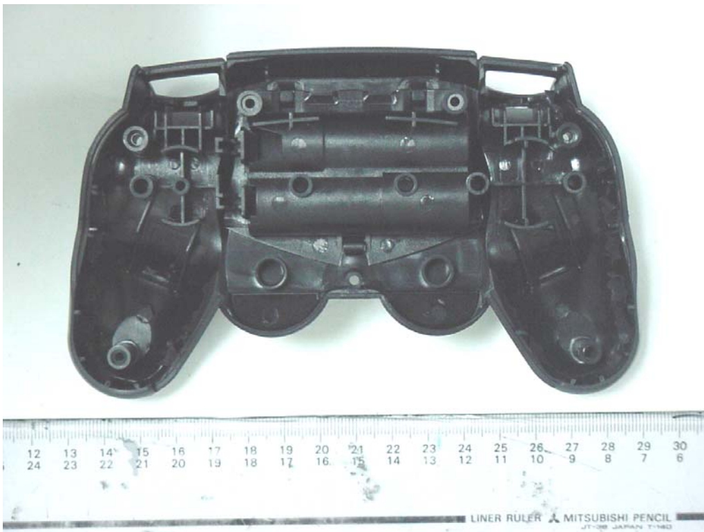
Game Controller – Bottom Housing Internal View
