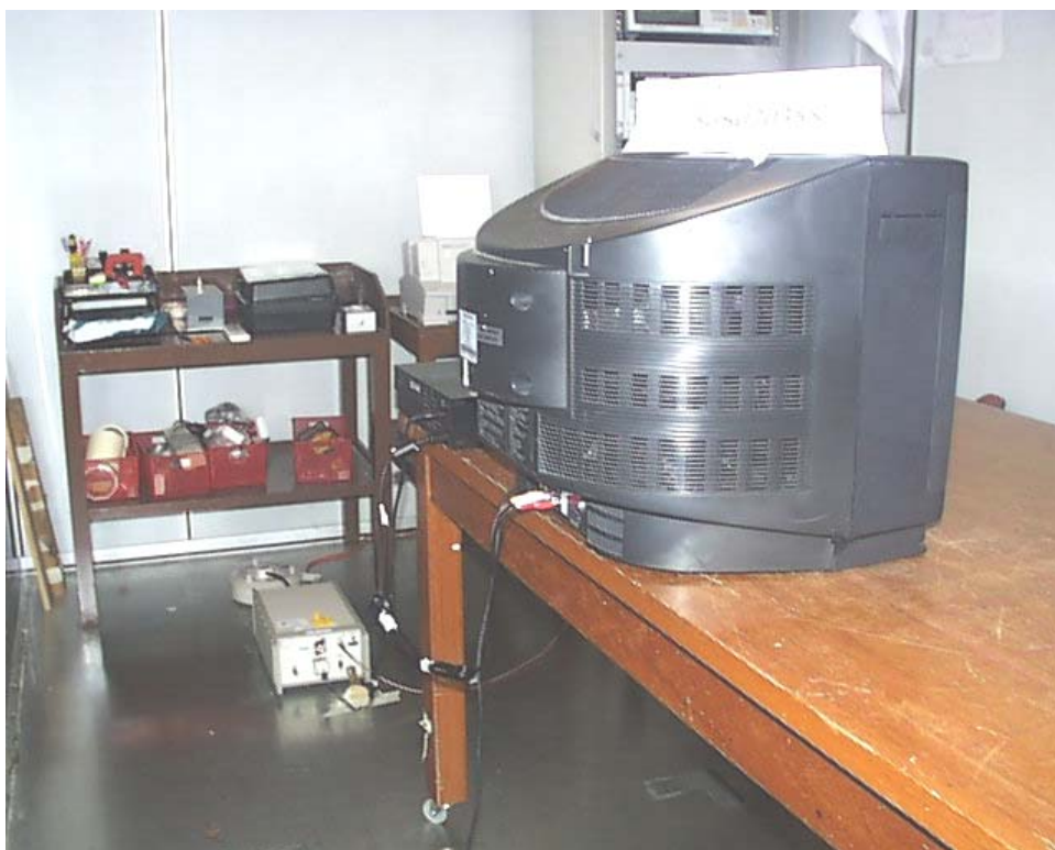
Conducted Emissions Setup (Rear View)
