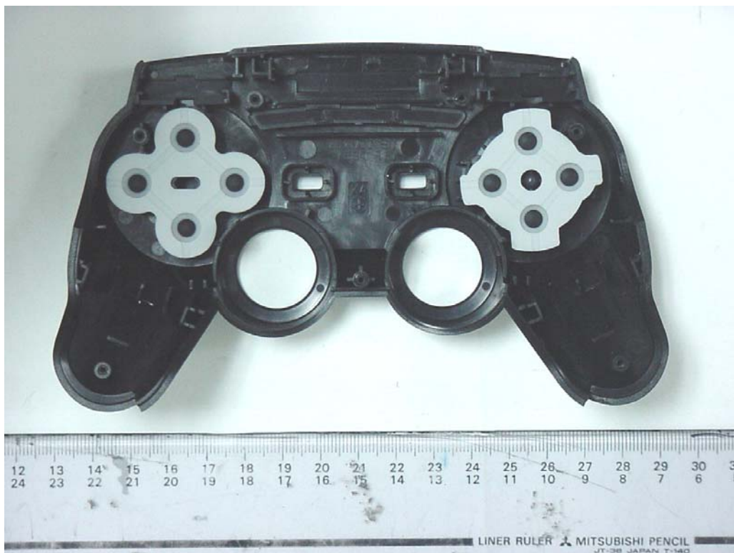
Game Controller – Top Housing Internal View
