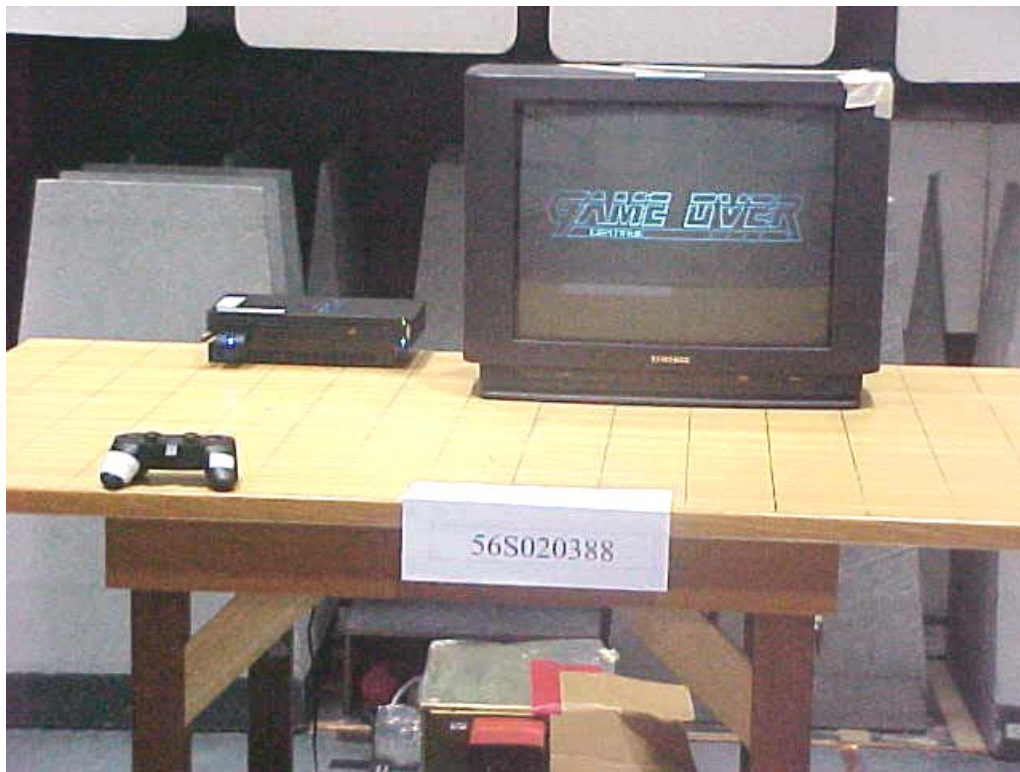
Radiated Emissions Setup (Front View)
