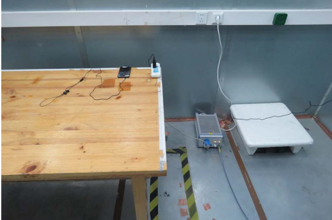
Picture 3 Conducted Emission Test Setup
