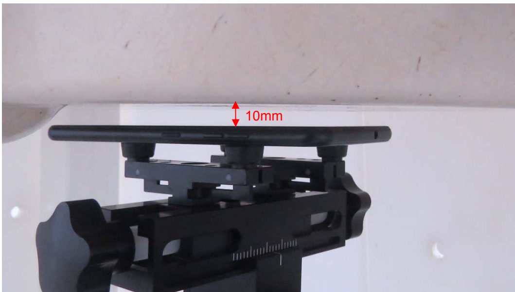
Picture 13: Front Side, the distance from handset to the bottom of the Phantom is 10mm
