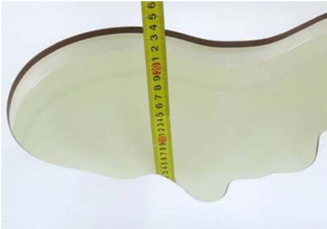
Picture 3: Liquid depth in the head Phantom (5250 MHz, 15.4cm depth)
