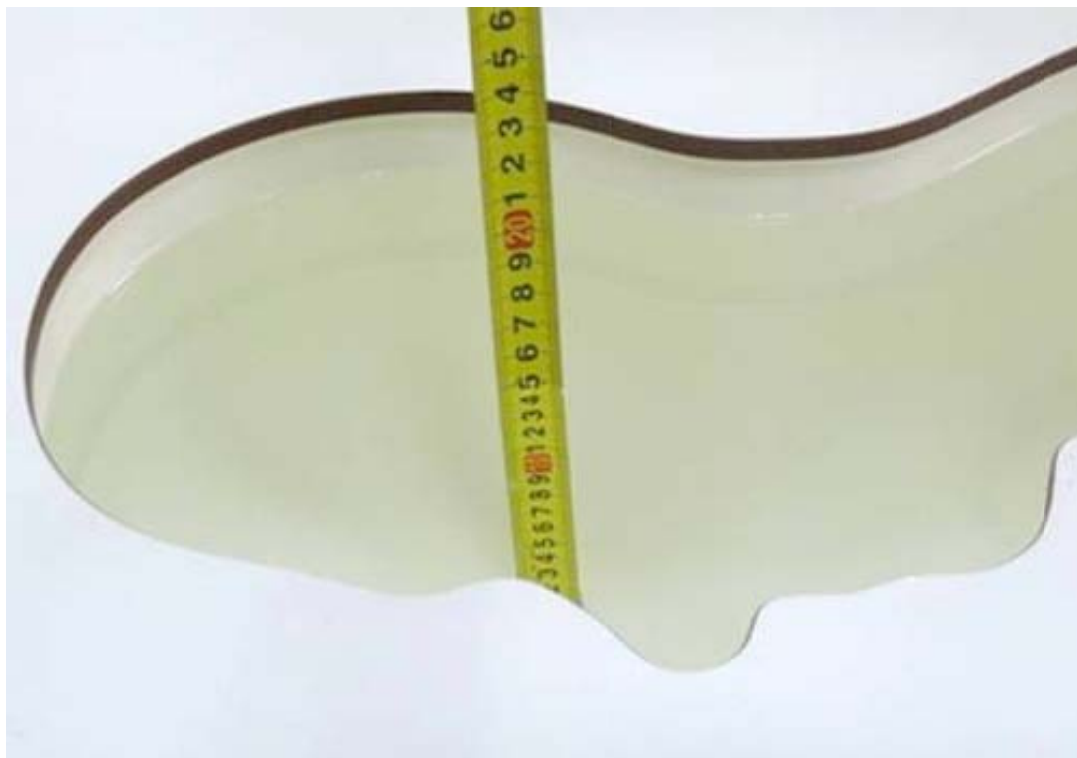
Picture 5: Liquid depth in the head Phantom (5750 MHz, 15.1cm depth)
