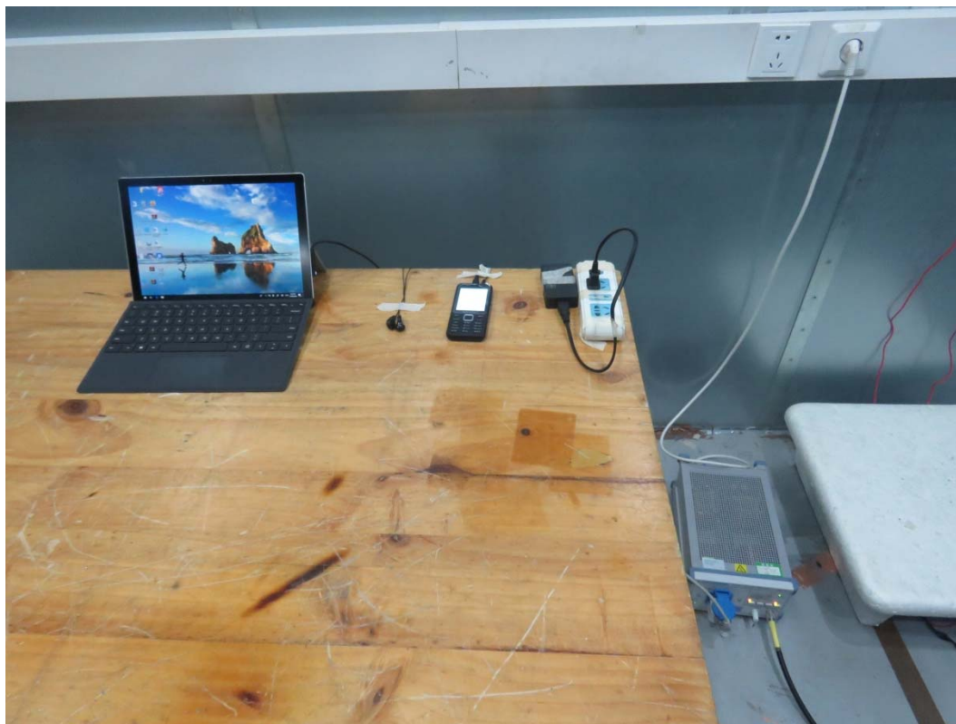
Picture 2 Conducted Emission Test Setup
