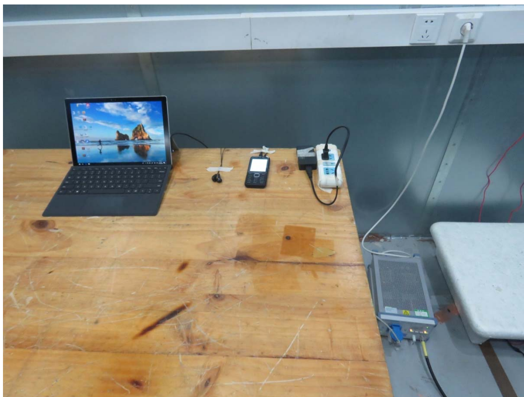
Picture 2 Conducted Emission Test Setup
