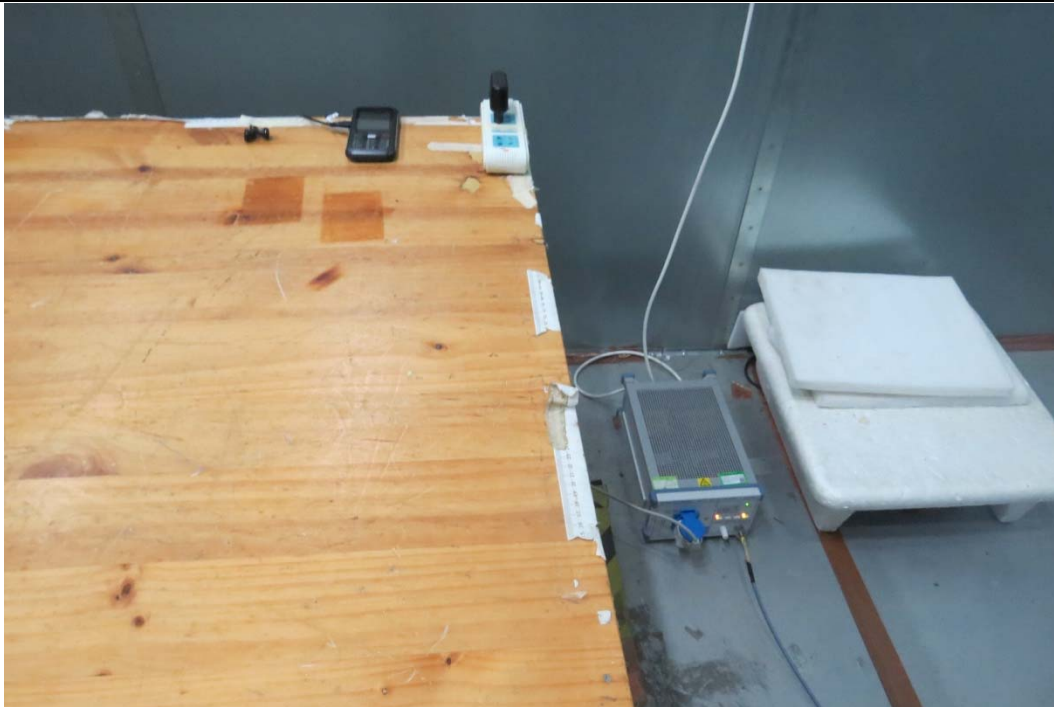
Picture 3 Conducted Emission Test Setup
