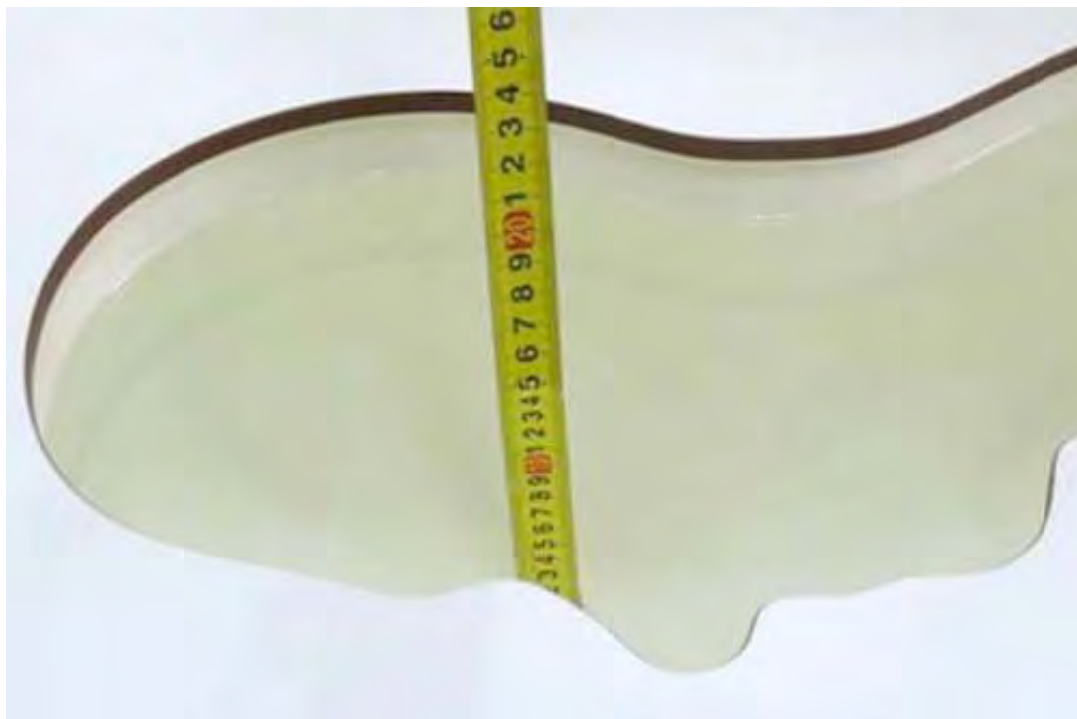
Picture 3: liquid depth in the head Phantom
