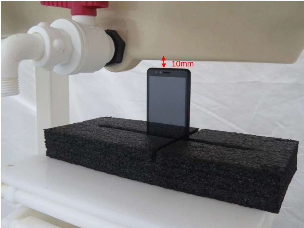
Picture 11: Top Side, the distance from handset to the bottom of the Phantom is 10mm
