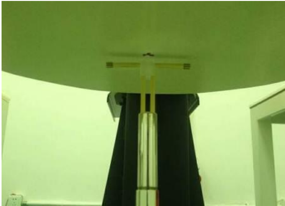
Picture 8.2 Photo of Dipole Setup
