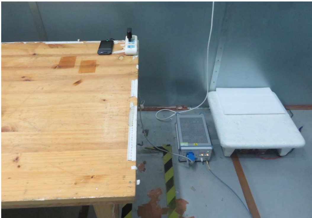
Picture 3 Conducted Emission Test Setup
