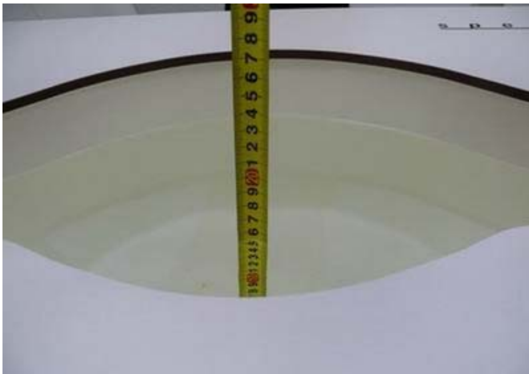
Picture 3: Liquid depth in the flat Phantom
