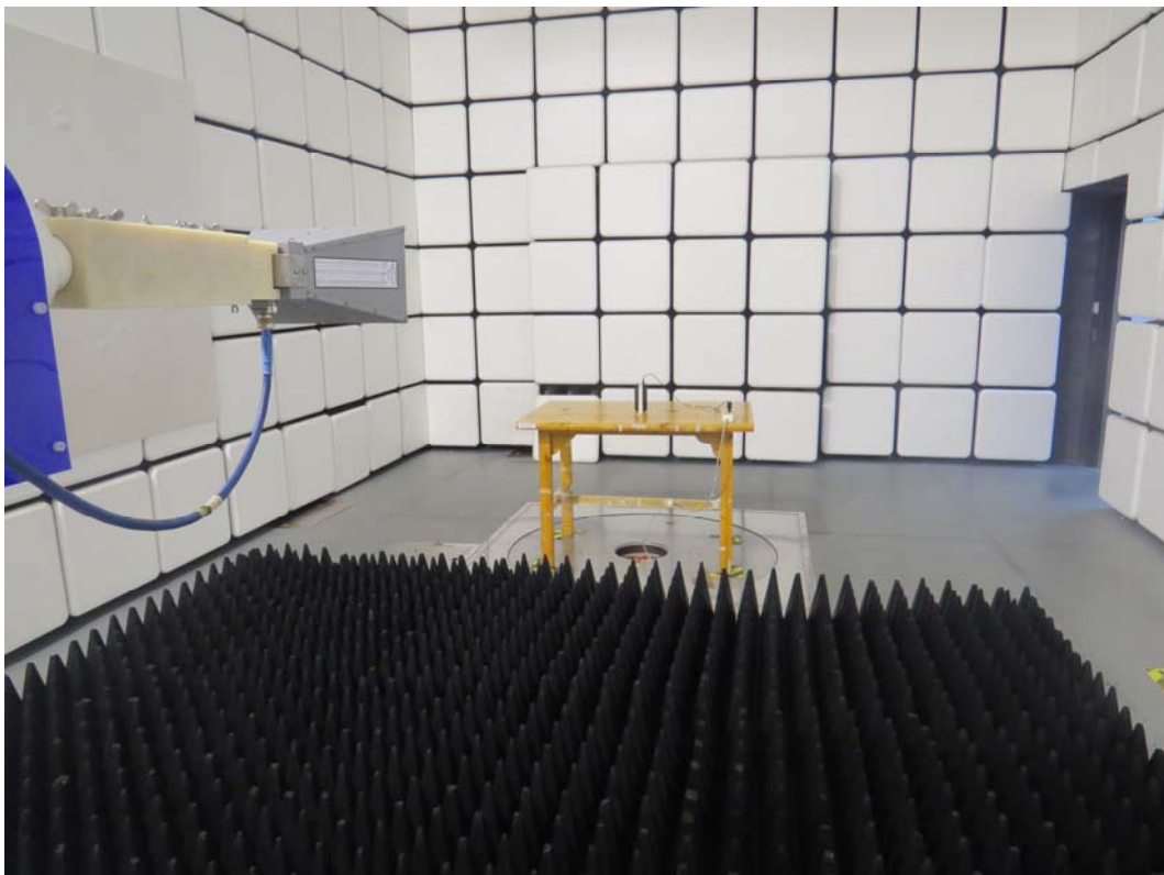
Picture 2: Radiated Spurious Emissions Test setup
