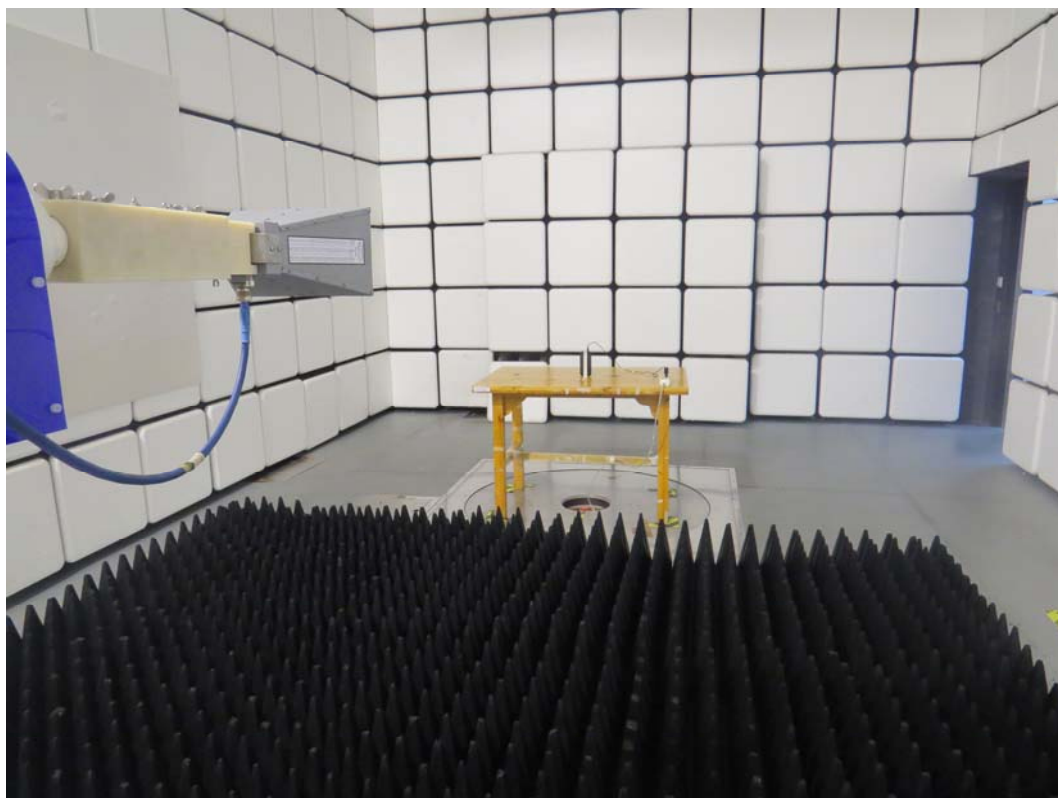
Picture 2: Radiated Spurious Emissions Test setup
