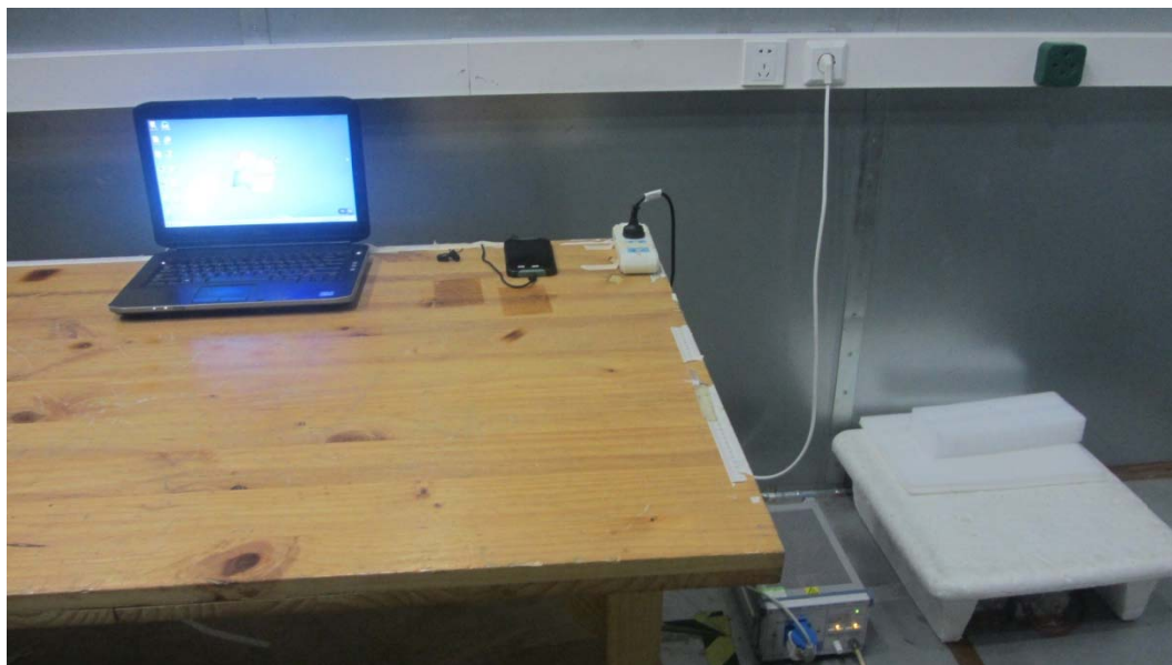
Picture 3 Conducted Emission Test Setup
