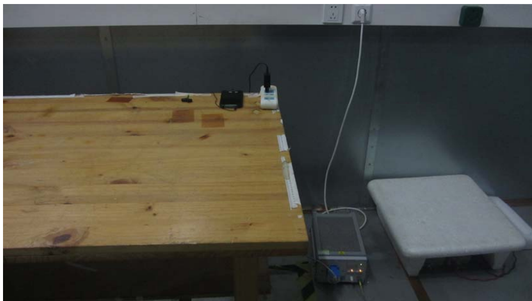
Picture 3 Conducted Emission Test Setup
