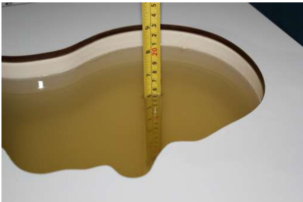
Picture 7-4: Liquid depth in the Head Phantom(2550MHz)
