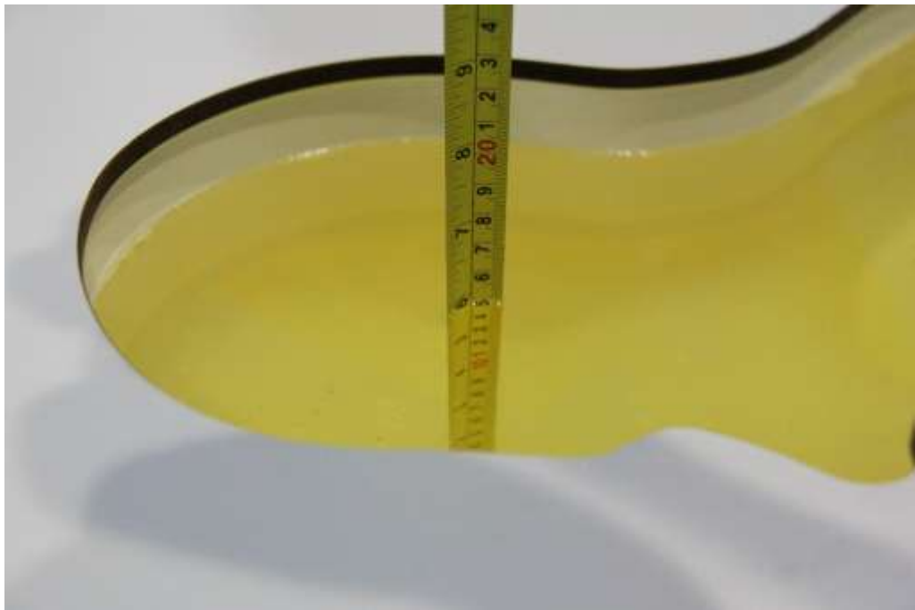
Picture 7-3: Liquid depth in the Head Phantom(2450MHz)
