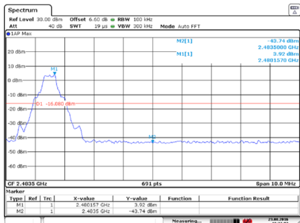
BT DH5 CH78, Carrier frequency (MHz): 2480
