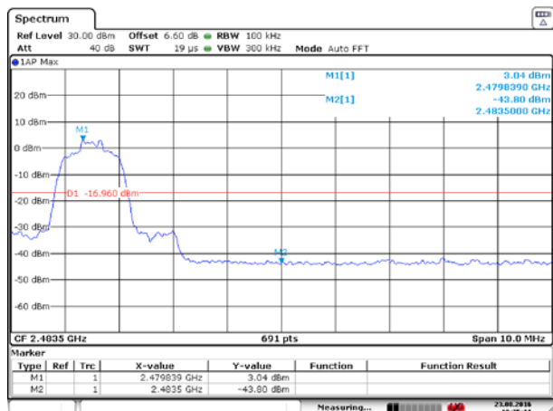
BT 2DH5 CH78, Carrier frequency (MHz): 2480
