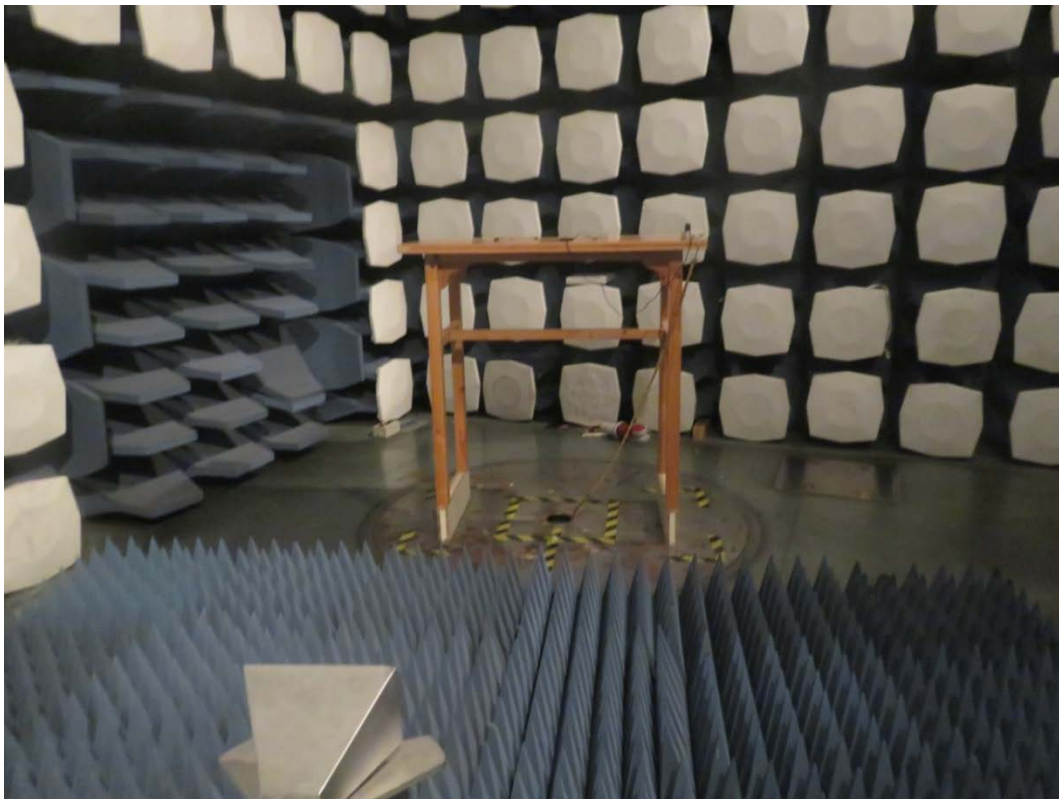
Picture 2 Radiated Emission Test Setup
