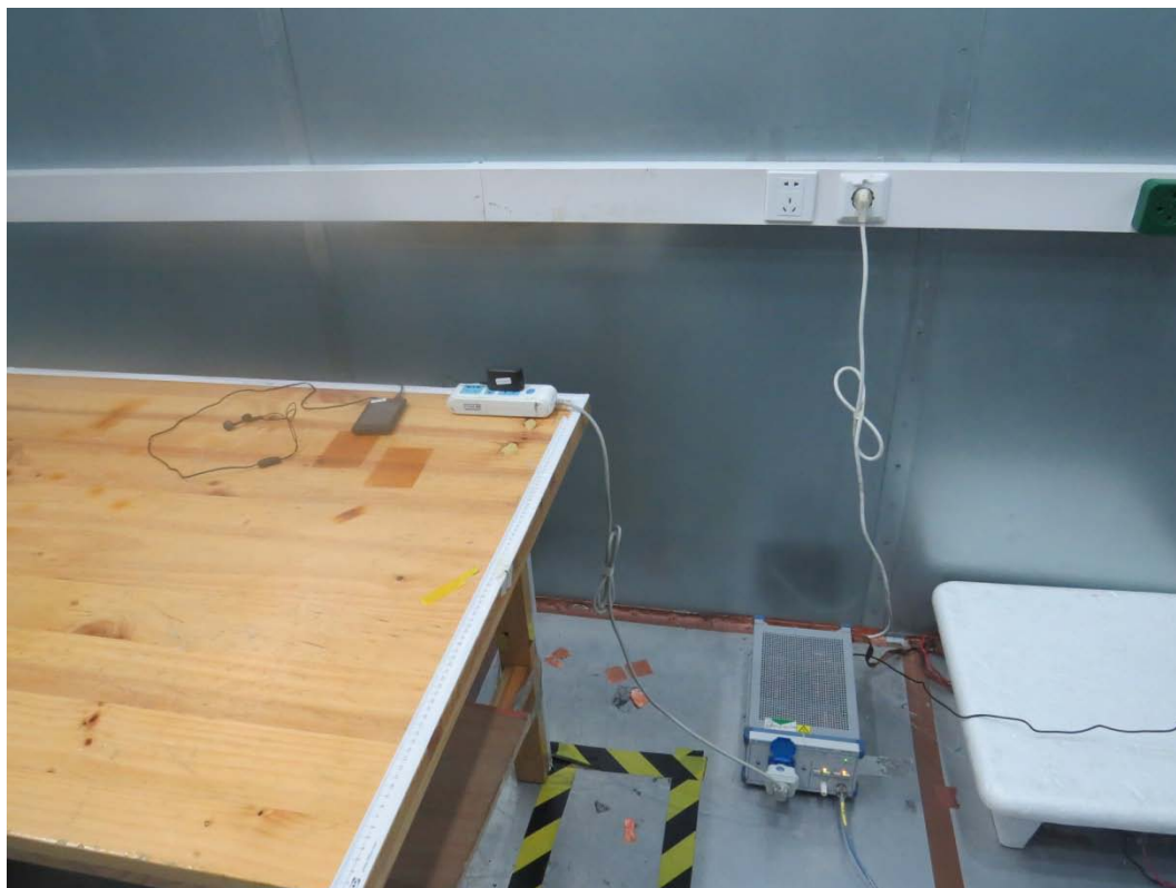
Picture 3 Conducted Emission Test Setup
