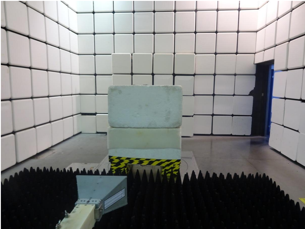
Picture 1: Radiated Spurious Emissions Test setup
