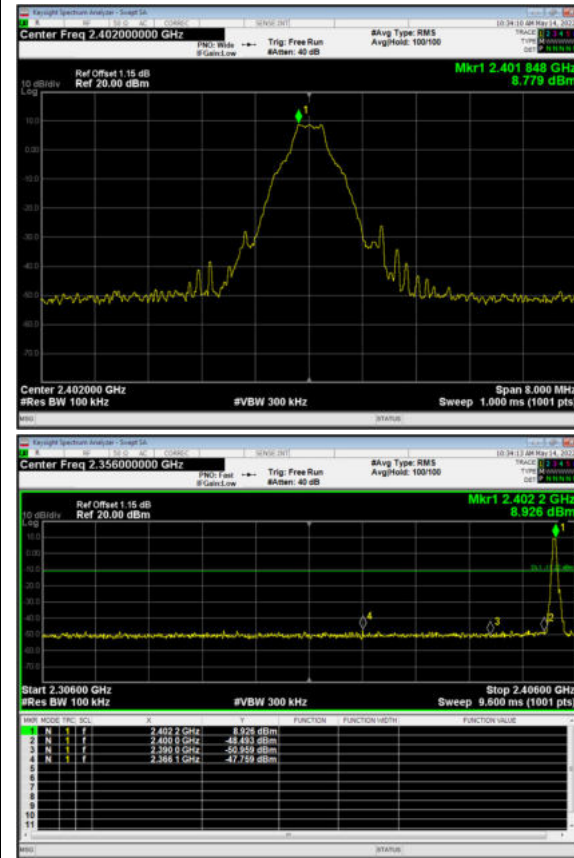
BT DH5 CH0, Carrier frequency (MHz): 2402
