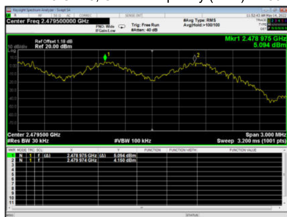
BT DH5 CH78, Carrier frequency (MHz): 2480
