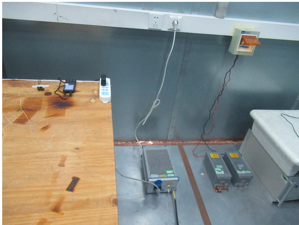
Picture 2 Conducted Emission Test Setup
