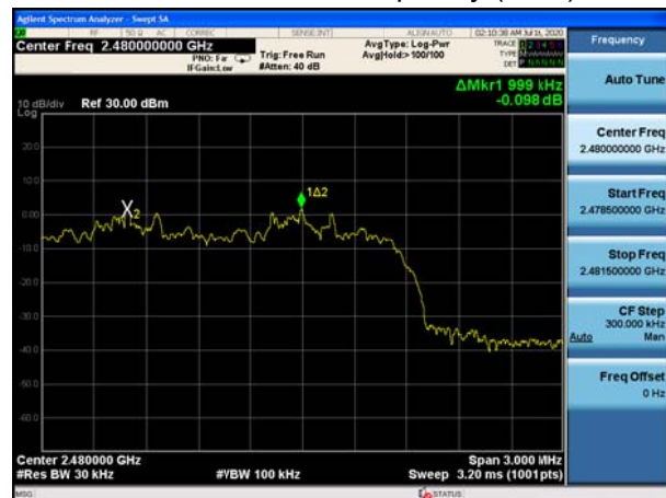
BT 2DH5 CH78, Carrier frequency (MHz): 2480
