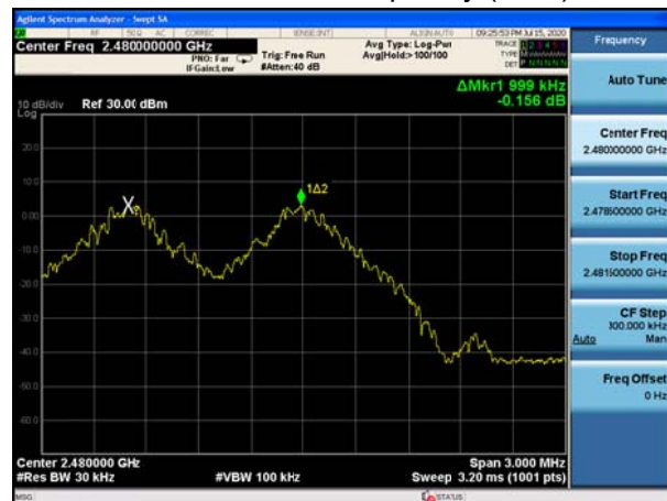
BT DH5 CH78, Carrier frequency (MHz): 2480
