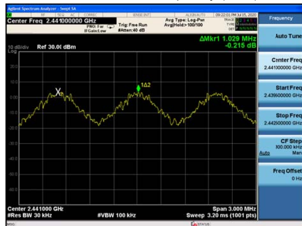
BT DH5 CH78, Carrier frequency (MHz): 2480
