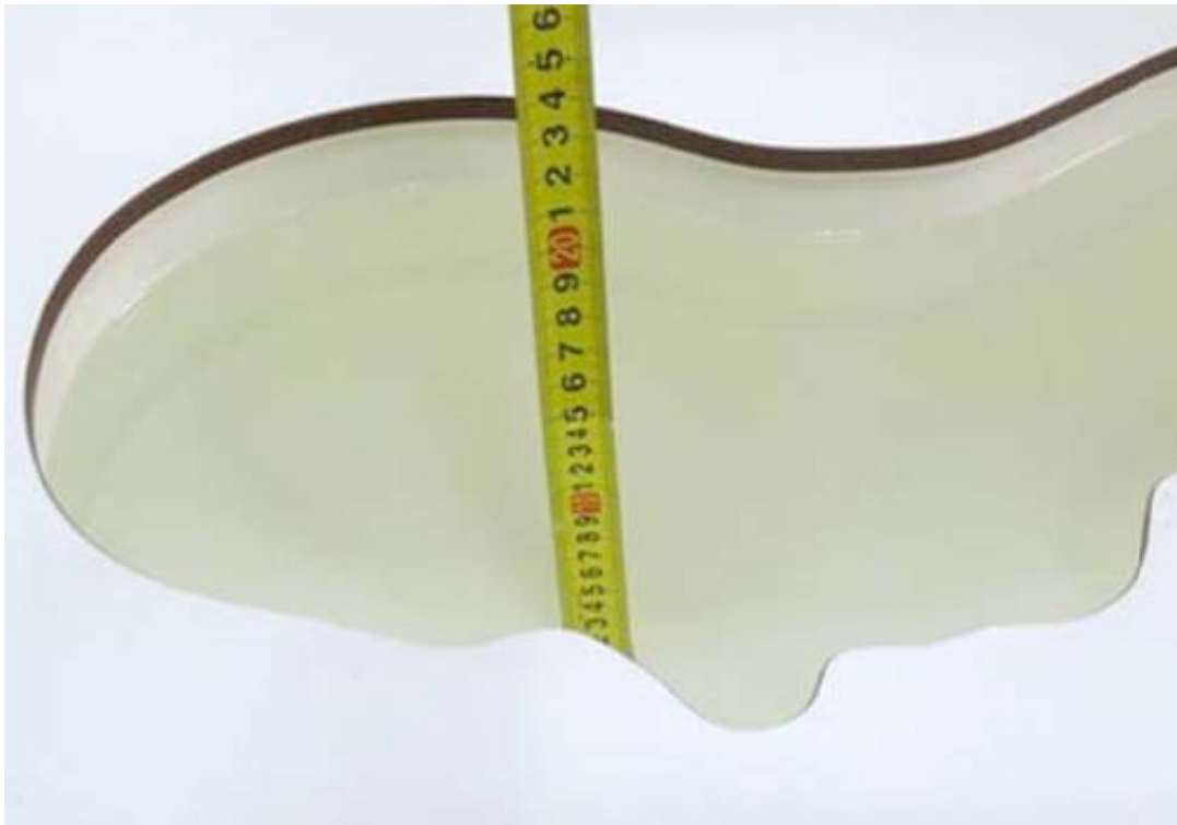
Picture 6: liquid depth in the head Phantom (1900 MHz, 15.3cm depth)
