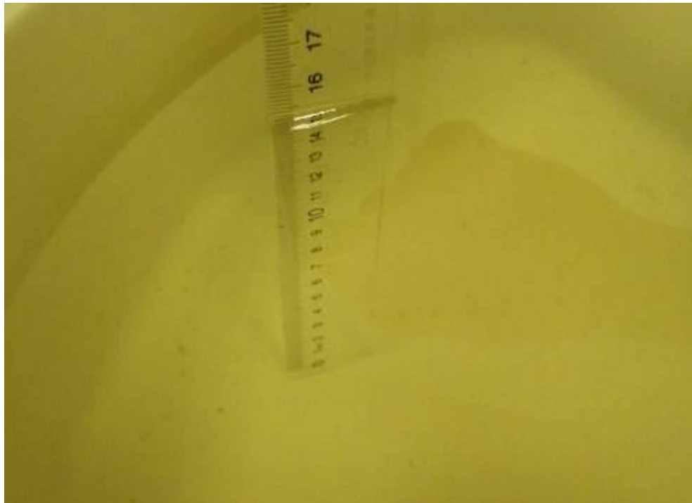
Picture 7-1: Liquid depth in the Flat Phantom (835 MHz Body)
