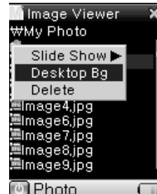
(Figure 32-2) To set the image as background of main menu, select an image and press button (M) and press button (PLAY/OFF ) in main menu.
