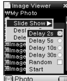
(Figure 32-1) When press button (M) in image viewer, main menu is displayed. To consecutively play big images, check time in figure 32-1 and select START>
