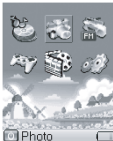
(Figure 31-1) In Start screen, move to Image viewer icon. And then press button (PLAY/OFF) and Image viewer window of figure 31-2 is displayed.
