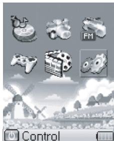
(Figure 39-1) Move to CONTROL icon in Start menu and press button (PLAY/OFF ). Control menu window of figure 39-2 is displayed.
