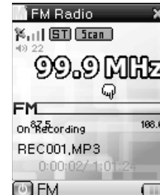
(Figure 34-3) When holding down ( ) long during radio play, recording begins as figure 34-3. To stop recording, press button (REC ) again.
