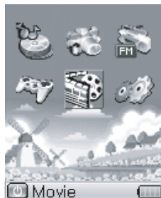
(Figure 37-1) Move to Movie Player in Start menu figure 37-1, press button (PLAY/OFF). Movie player window of figure 37-2 is displayed and saved movie file is played.
