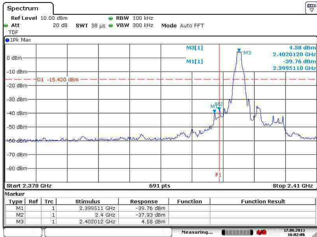
Figure 16. Conducted emission at low band edge.
