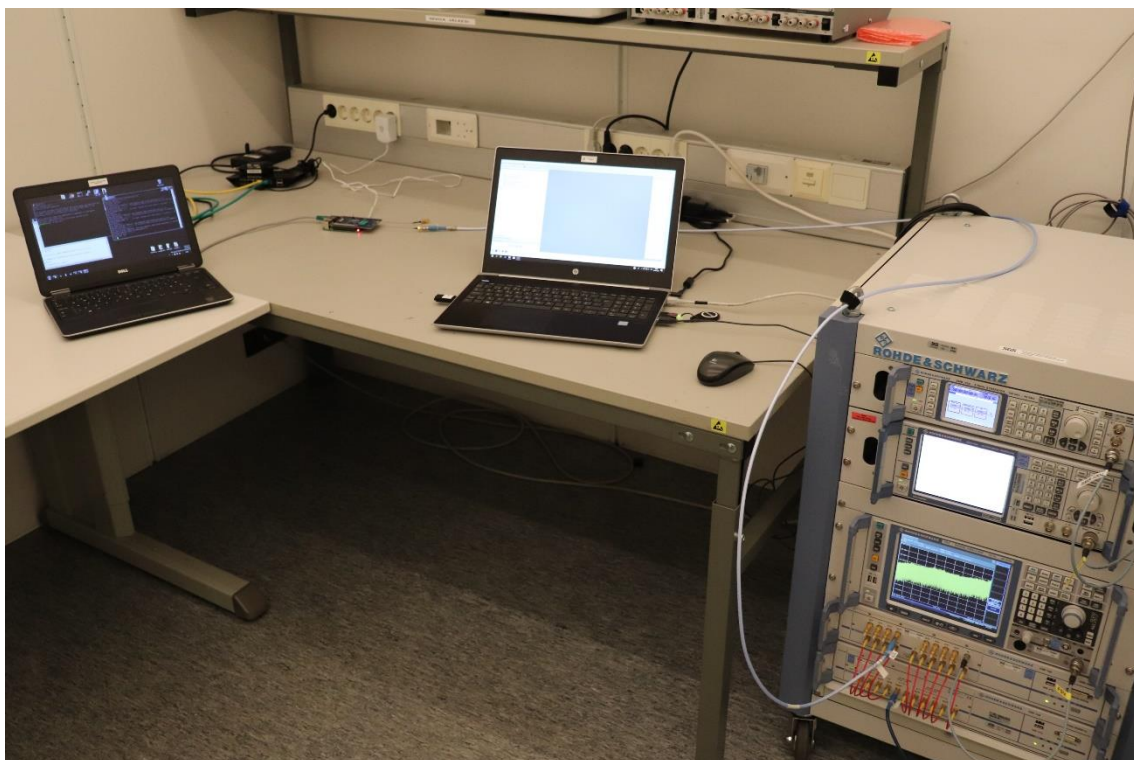
Photograph 12. FCC Conducted measurement
