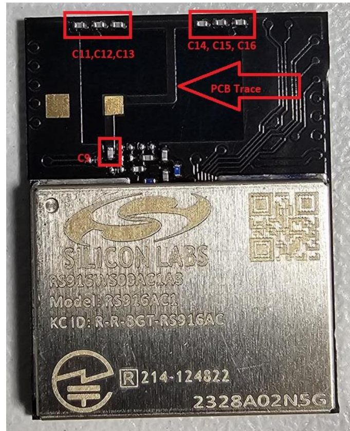
Figure 7: Photo of the antenna realized on the RS916AC1. It consists of a PCB antenna trace and 7 ceramic capacitors (C9,C11-C16)
