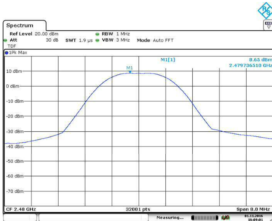
Figure 1: Conducted power (ch high)
